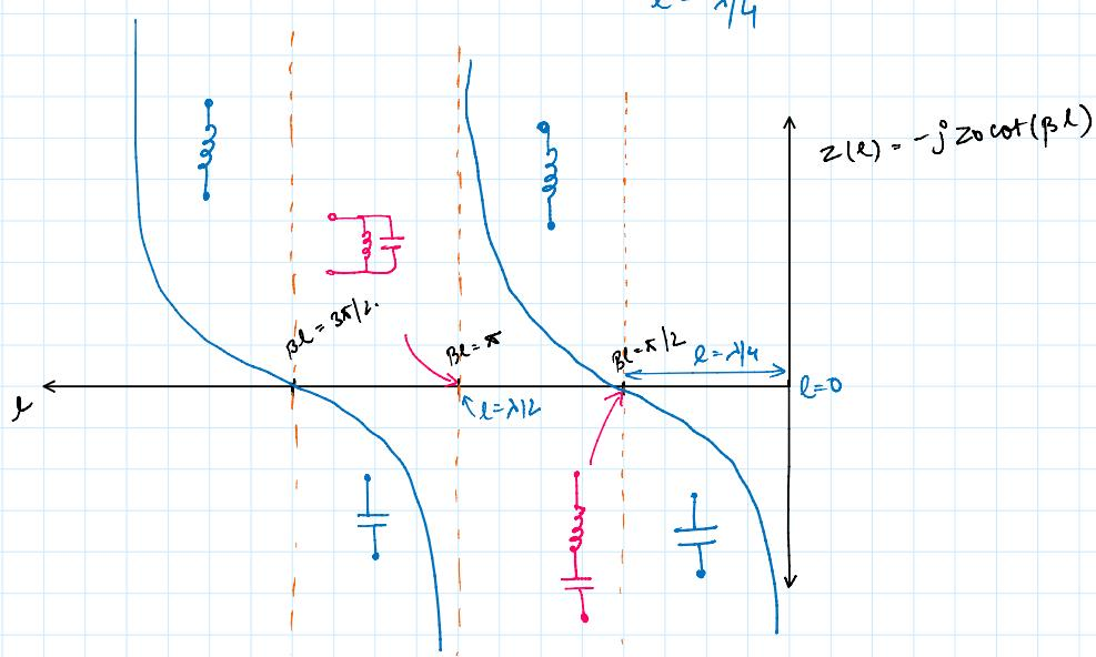
$$\begin{aligned} \bullet & \quad 0 \leq l < \lambda/4 \quad \equiv \quad \frac{1}{T} \\ \bullet & \quad \frac{\lambda}{4} < l < \frac{\lambda}{2} \quad \equiv \quad \text{---} \\ \bullet & \quad \frac{\lambda}{2} < l < 3\lambda/4 \quad \equiv \quad \frac{1}{T} \\ & \quad \vdots \end{aligned}$$
