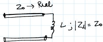
$$|\Gamma_L| = 1 \quad \Gamma_L = \frac{Z_L - Z_0}{Z_L + Z_0} = \frac{j\omega L - Z_0}{j\omega L + Z_0}$$
