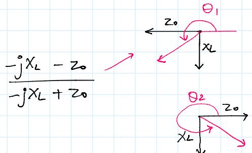
$-\pi < \angle Z_L < 0$  Capacitive load.
