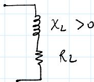
$$\underline{\Gamma}_L = \frac{R_L + jX_L - Z_0}{R_L + jX_L + Z_0}$$
