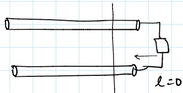
$$Z(e) = \text{real} = \frac{V(e)}{I(e)} \quad \text{when } \angle \Gamma_i = 0^\circ \text{ or } 180^\circ$$
