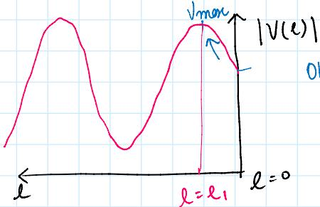
Observation: Starting from load towards generator, we first hit  $V_{max}$ .
