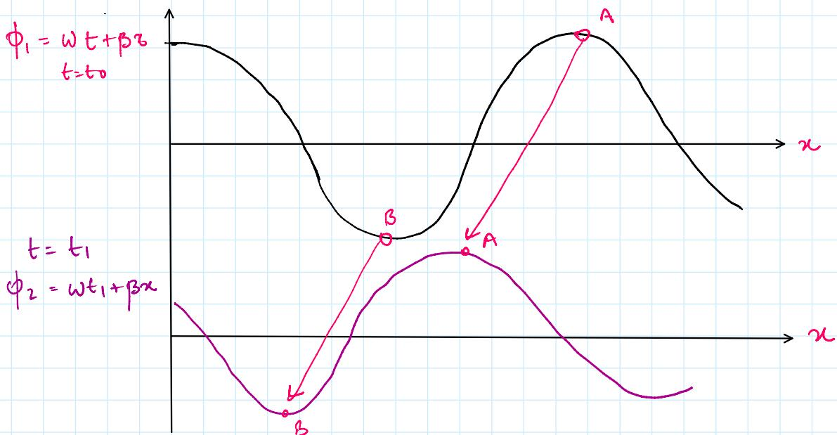
$$\text{Propagation Constant : } \gamma = \sqrt{(R+j\omega L)(G+j\omega C)} = \underline{\alpha} + j\underline{\beta}$$
