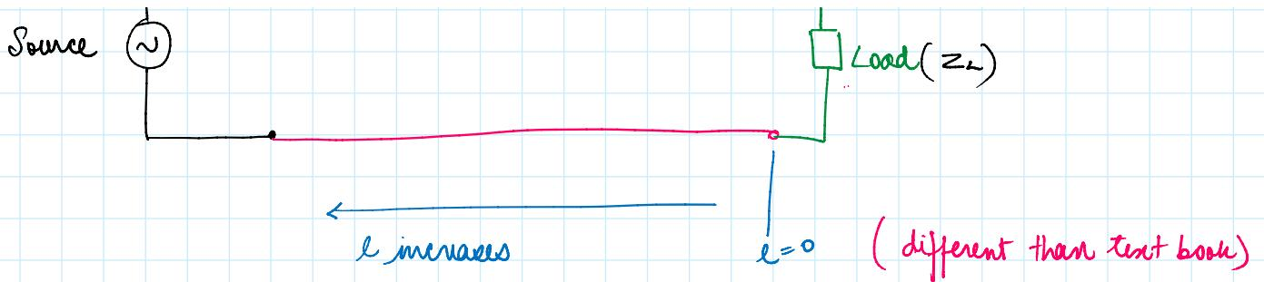
$$\left. \begin{aligned} V &= V^+ e^{rl} + V^- e^{-rl} \\ I &= I^+ e^{rl} + I^- e^{-rl} \end{aligned} \right\} \quad (1) \quad (2)$$
