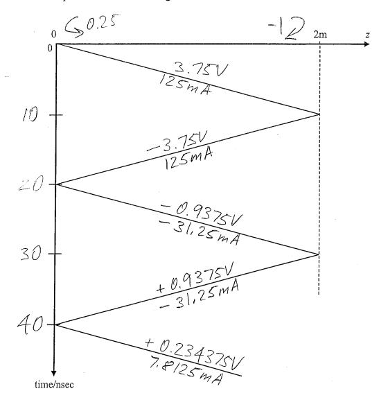
(h) Determine the voltage at the input of the coaxial cable,  $v_{in}$ , at time t = 45nsec.
