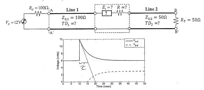
(a) Determine the delay times of line 1 and line 2, respectively.
