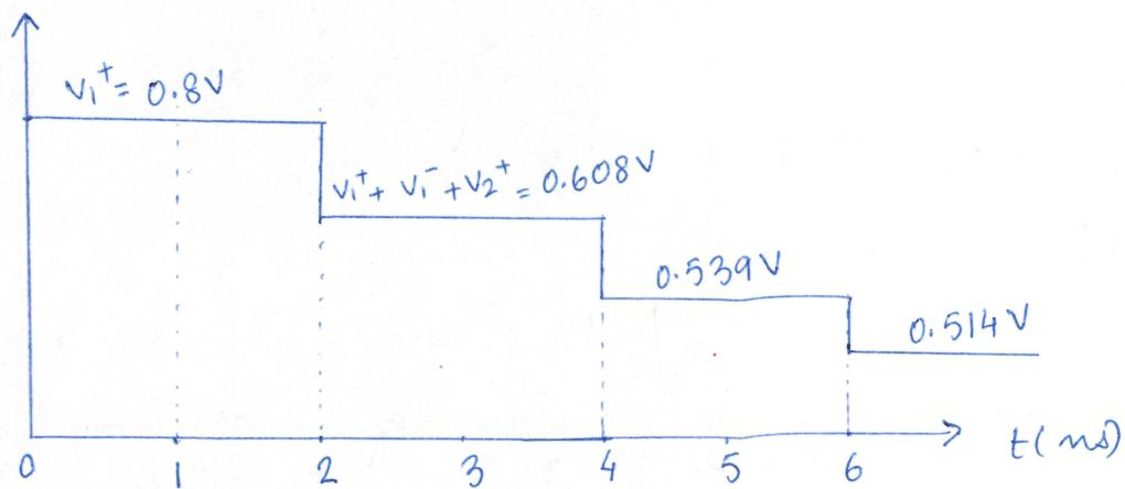
**Problem 4: (20 points)** Given the following transmission line and measurement of voltage near generator  $V_A(t)$ :
