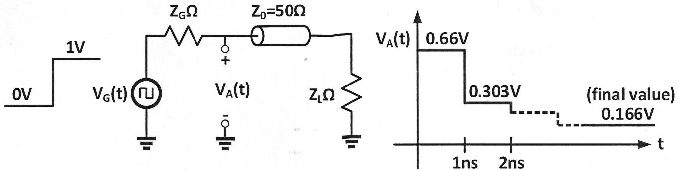
(a) (14 points) Calculate the impedance  $Z_G$  and  $Z_L$ .
