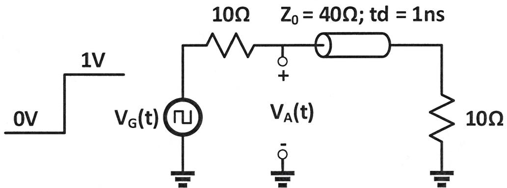
(a) (5 points) Calculate the reflection coefficient at the generator side and load side:
