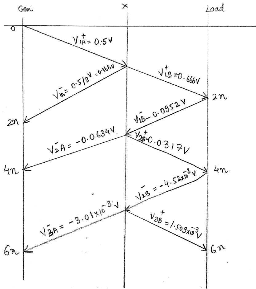
(b) (5 points) Draw waveform of voltage on node X versus time for up to 6ns.
