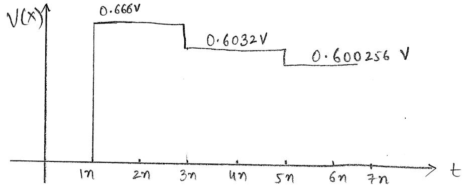
**Problem 4: (15 points)** A transmission line with characteristic impedance of  $Z_0=50\Omega$  is terminated with an un-known load impedance  $Z_L$ . The voltage standing wave pattern along the transmission line as a function of distance is shown below.
