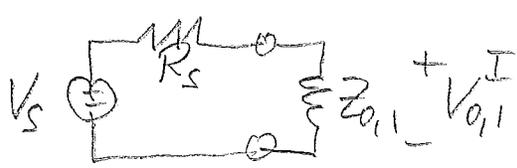
$$\Rightarrow V_s = V_{0,1}^I \frac{z_{0,1} + R_s}{z_{0,1}} = 30V \frac{90 + 45}{90} = \boxed{45V}$$
