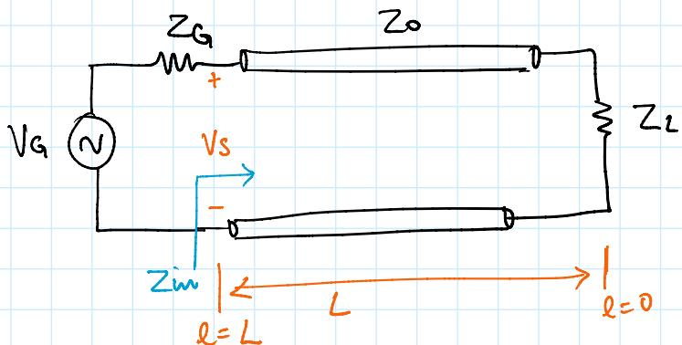
$$V(l) = V^+ e^{j\beta l} \left( 1 + |Y_L| e^{j(\phi_L - 2\beta l)} \right) \quad \left. V_S = V(l) \right|_{l=L} = V^+ e^{j\beta L} \left( 1 + |Y_L| e^{j(\phi_L - 2\beta L)} \right) \quad -(1)$$
