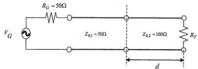
(a) What is the physical length of the  $100\Omega$  line if  $f = f_0 = 200 \,\text{MHz}$  and the effective dielectric constant of the transmission line is  $\varepsilon_{r,eff} = 4$ ?
