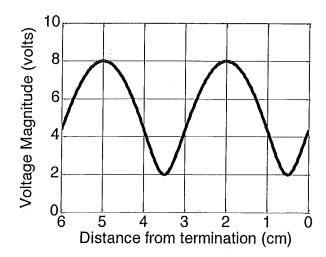
(a) What is the standing-wave ratio on the line terminated in the unknown load impedance  $Z_L$ ?
