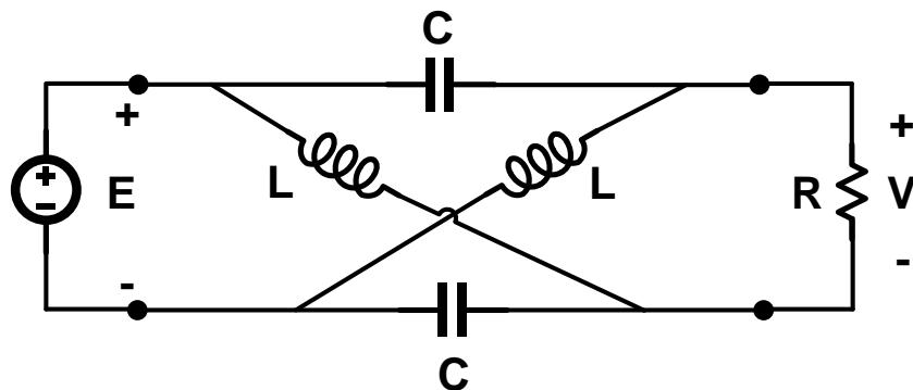
Q2: Calculate the transmission zero of the following network.
