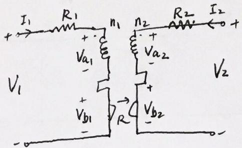
$$\left\{ \begin{array}{l} Y_{11} = \frac{I_1}{V_1} \Big|_{V_2=0} \\ V_1 = I_1 R_1 + V_{a1} + V_{b1} \\ V_{a1} = \frac{n_1}{n_2} V_{a2} \\ V_{b1} = -R I_2 \\ I_2 = -\frac{n_1}{n_2} I_1 \end{array} \right.$$
