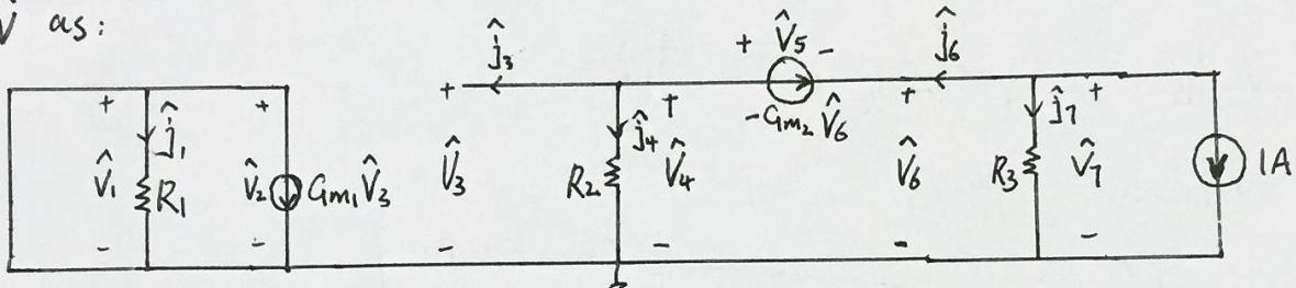
$$\text{In } N: \quad V_1 = V_2 = V_{in}. \quad V_3 = V_4 = -G_{m1} R_2 V_{in}. \quad V_5 = -\frac{G_{m1} R_2 V_{in}}{1 + G_{m2} R_3}. \quad V_6 = V_7 = -\frac{G_{m1} G_{m2} R_2 R_3 V_{in}}{1 + G_{m2} R_3}$$
