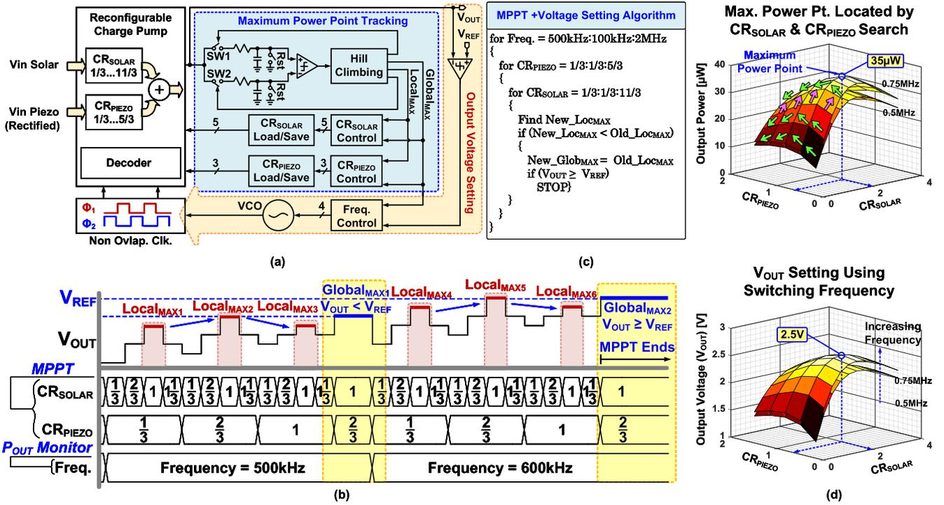
Fig. 5. (a) Proposed MPPT and output voltage control architecture. (b) Timing diagram of the proposed algorithm. (c) Pseudo code of the proposed algorithm. (d) Simulated output power and voltage versus  $CR_{PIEZO}$  and  $CR_{SOLAR}$  for two switching frequencies 0.5 MHz and 0.75 MHz.
