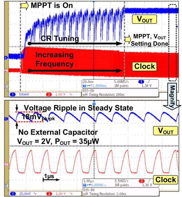
Fig. 13. Measured MPPT transient and steady state output voltage ripple.
