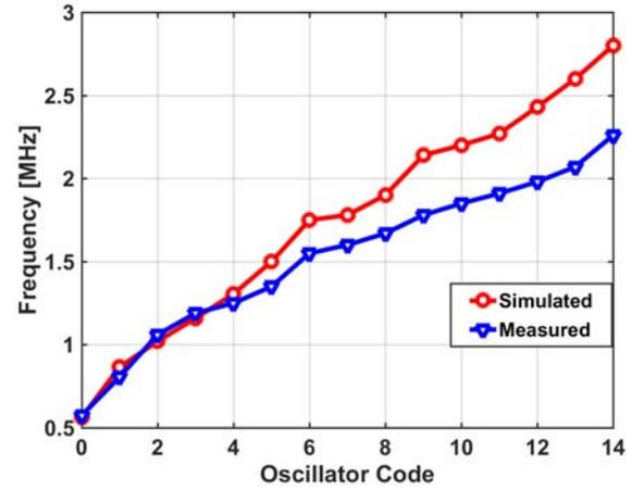
Fig. 15. Measured and simulated oscillator frequency versus oscillator digital code.
