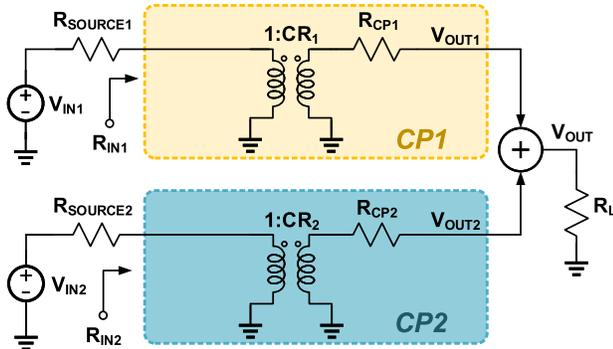
Fig. 2. Pseudo-static model of the proposed switched capacitor with dual input single output.
