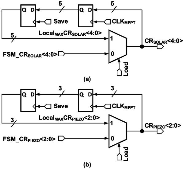
Fig. 9. Schematic of load and save registers for (a) solar conversion ratio and (b) piezo conversion.
