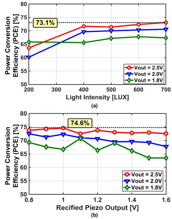
Fig. 16. (a) Measured power conversion efficiency versus light intensity. (b) Measured power conversion efficiency versus rectified piezo voltage.
