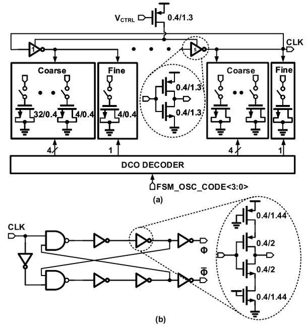
Fig. 7. (a) Digitally controlled ring oscillator. (b) Non-overlapping clock generator.
