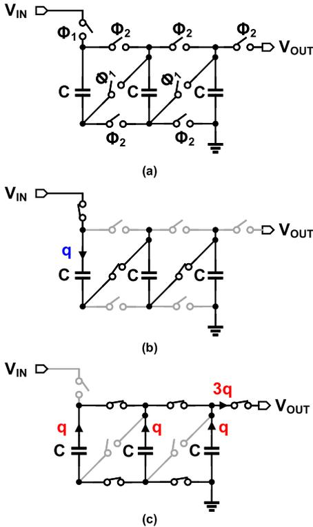
Fig. 4. (a) Series-parallel charge pump architecture with 1/3 conversion ratio. (b) Charge pump configuration during phase  $\Phi_1$ . (c) Charge pump configuration during phase  $\Phi_2$ .
