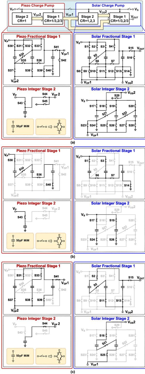
Fig. 6. (a) Proposed charge pump architecture with integer and fractional stages. (b) Charging phase ( $\Phi_1$ ) configuration for  $CR_{SOLAR} = 8/3$  and  $CR_{PIEZO} = 4/3$ . (c) Discharging phase ( $\Phi_2$ ) configuration for  $CR_{SOLAR} = 8/3$  and  $CR_{PIEZO} = 4/3$ .
