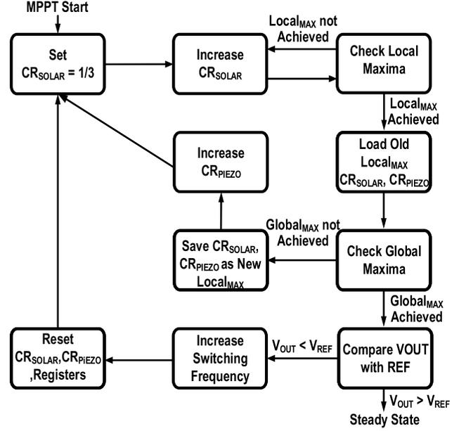
Fig. 10. Proposed finite state machine (FSM) for MPPT and output voltage setting.
