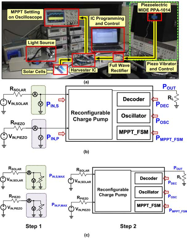
Fig. 12. (a) Energy harvester measurement setup. (b) Power measurements for power conversion efficiency (PCE) calculations. (c) Power measurements for end-to-end power efficiency ( $PE_{END-to-END}$ ) calculations.
