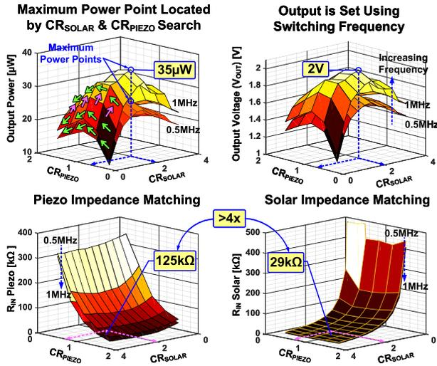
Fig. 14. Measured output power,  $CR_{SOLAR}$  and  $CR_{PIEZO}$  for  $V_{OUT} = 2$  V,  $R_{INT\ Solar} = 32$  k $\Omega$  and  $R_{INT\ Piezo} = 82$  k $\Omega$ .
