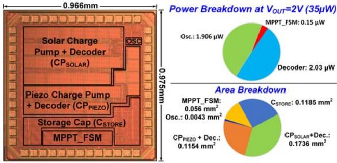
Fig. 11. Die micrograph of the proposed energy harvester, measured power breakdown at  $V_{OUT}=2V$  and area breakdown.
