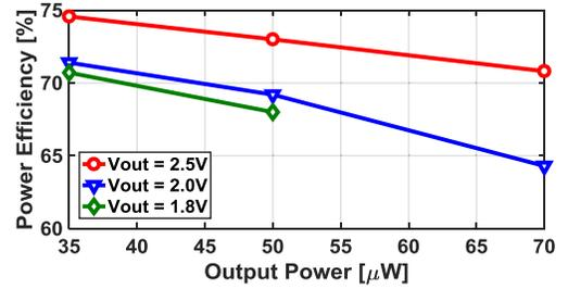
Fig. 18. Measured power conversion efficiency versus output power.
