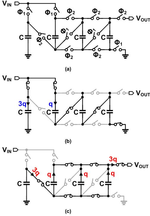
Fig. 3. (a) Series-parallel charge pump architecture with 4/3 conversion ratio. (b) Charge pump configuration during phase  $\Phi_1$ . (c) Charge pump configuration during phase  $\Phi_2$ .
