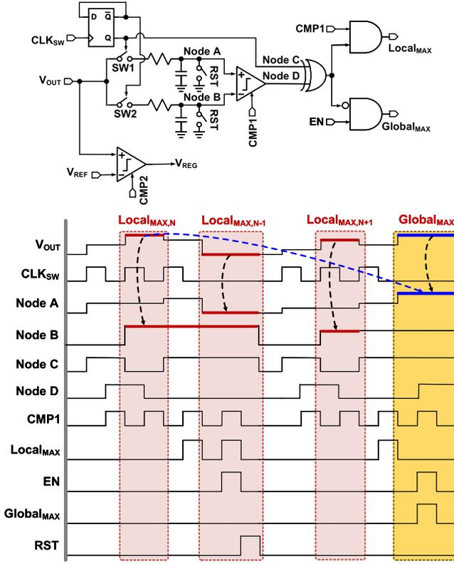
Fig. 8. Maximum power point tracking circuit and timing diagram.
