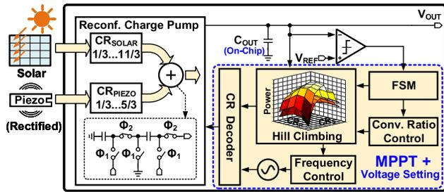
Fig. 1. Proposed multiple-input-single-output (MISO) switched capacitor based energy harvester concept with no external inductor or an external output capacitor.
