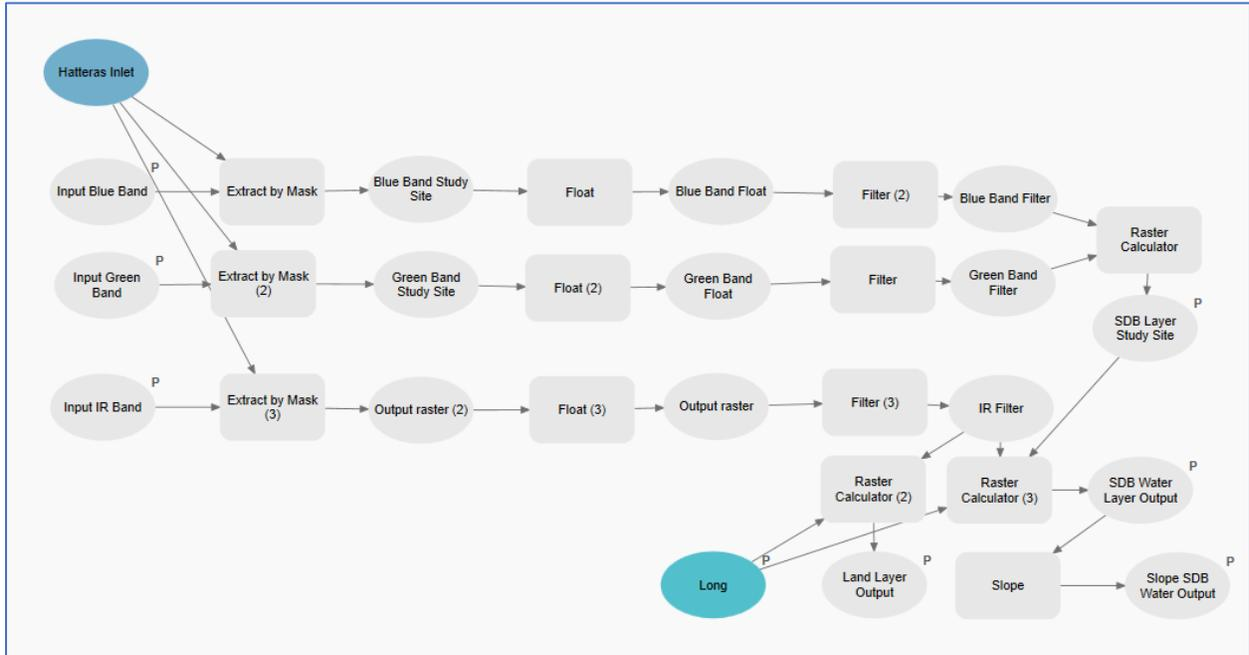
Image 3: The model builder above was created in ArcGIS Pro to perform the SDB workflow where the blue, green, and IR bands are utilized to create a water only SDB layer, a land layer, and slope layer of the SDB.
