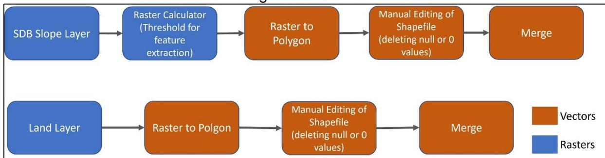
Image 8: Workflow and steps used for converting land and slope layers to vector data.
