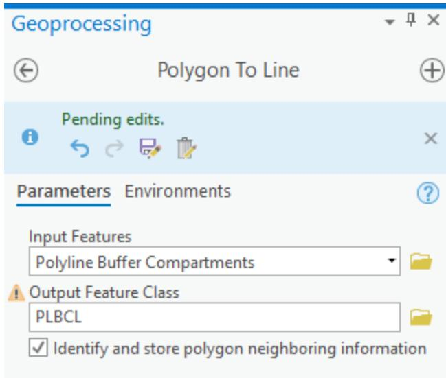
In order to extract cross sections, the polygon had to be separated into lines with the “Polygon to Line” tool. Figure 19 summarizes the parameters. “PLBCL” stands for Polyline Buffer Compartment Lines. This tool separates the compartments at the vertices. Once this step was completed, an individual line can be chosen and under the “Feature Layer” tab then “Create Chart” then “Profile graph”. The cross section can be displayed.
