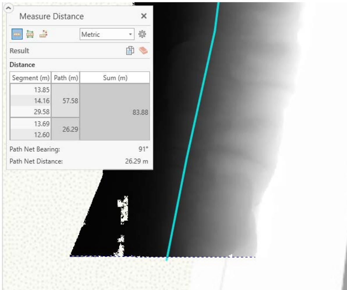
Figure 12: Use of measure tool to determine width of DEM at southern most segment of the DEM
