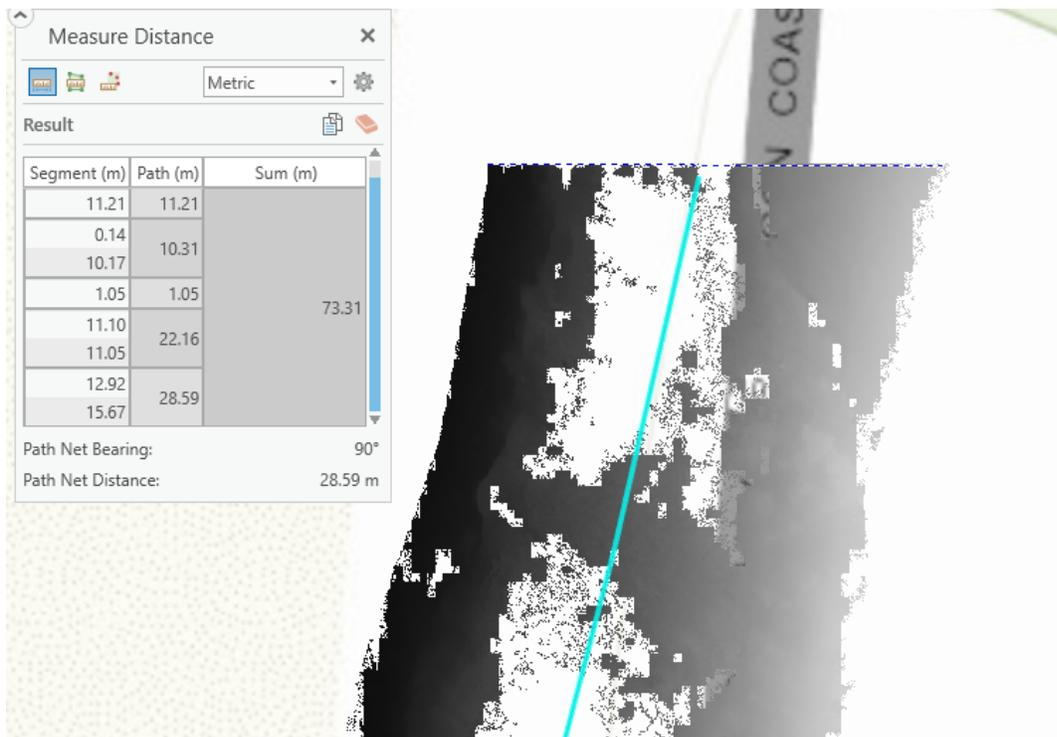
Figure 14: Use of measure tool to determine width of DEM at northern most segment
