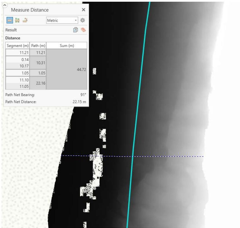
Figure 13: Use of measure tool to determine width of DEM at middle segment
