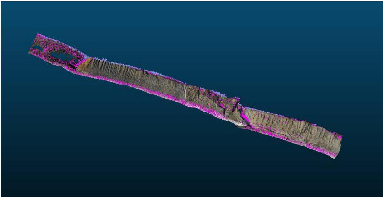
*Figure 8: Point cloud with holes filled*
