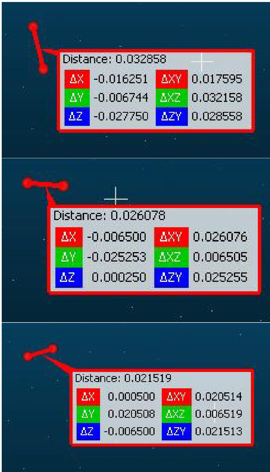
Figure 5: Point picking tool displaying multiple iterations to determine point spacing
