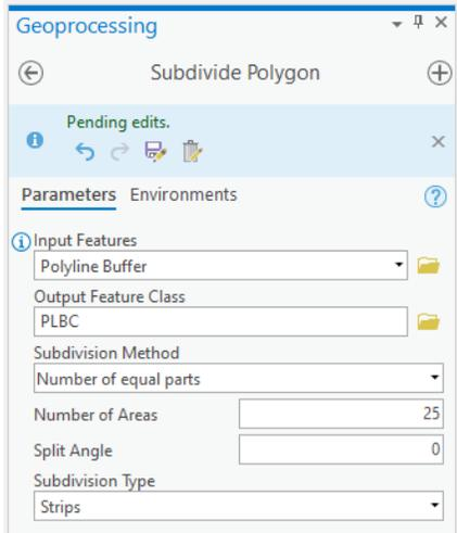
To create compartments, the “Subdivide Polygon” tool was used with the parameters outlined in Figure 17. “PLBC” stands for polyline buffer compartments. The subdivision method is “number of equal parts” with 25 equal parts shaped as “Strips”. When the polyline was drawn, 25 lines individual lines comprised the entire polyline. Therefore this value was an appropriate fraction to divide the entire buffer by. Figure 18 displays the map with the added polyline buffer compartments.
