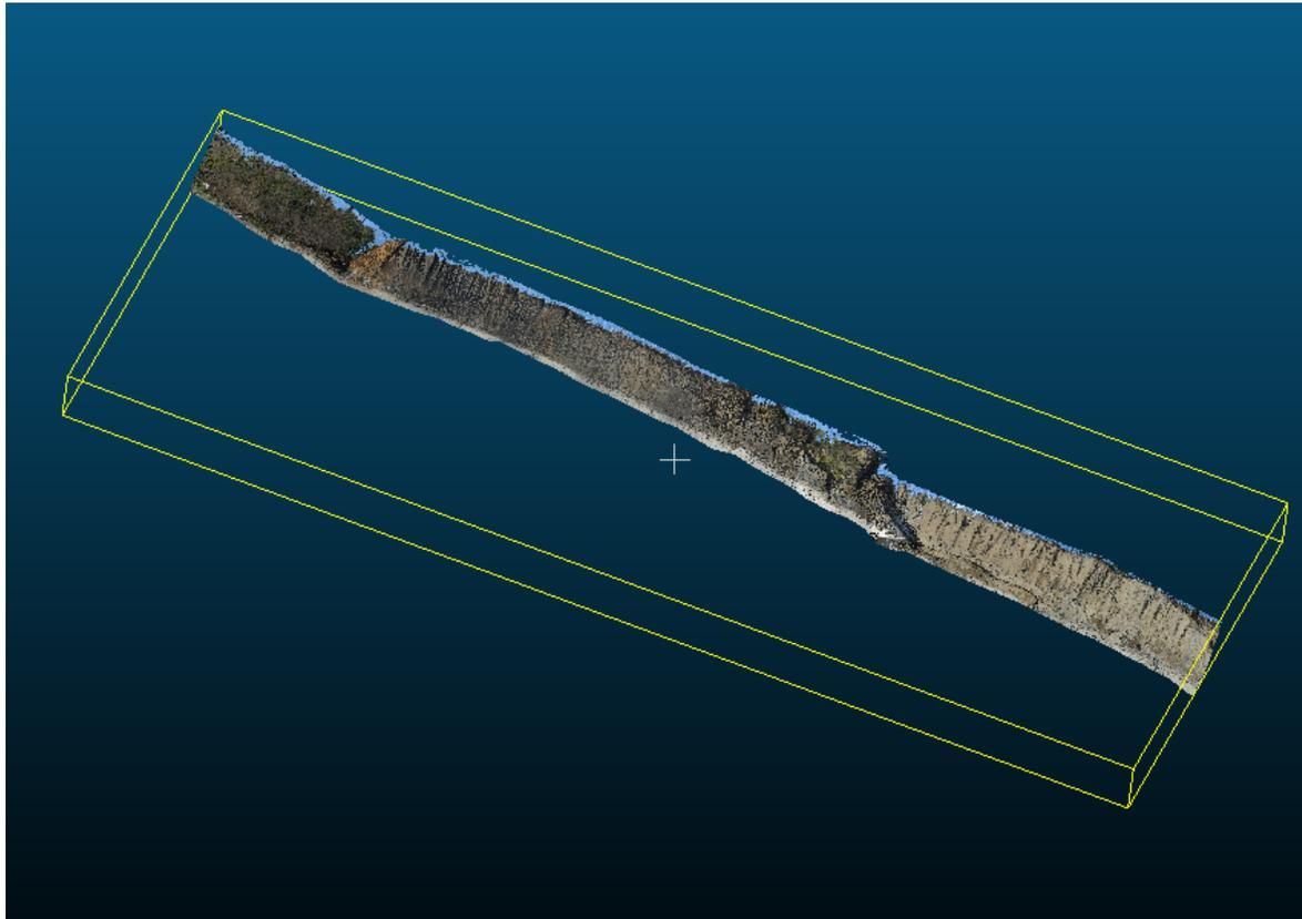
*Figure 4: Product of segment tool after removing all surfaces other than the sea cliff profile*
