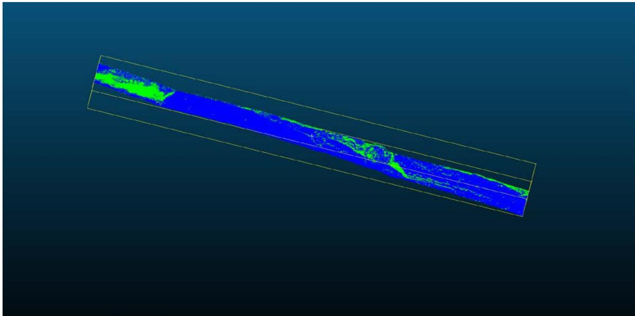
*Figure 6: Point Cloud Classified (or colored) separating ground points from non-ground points*
