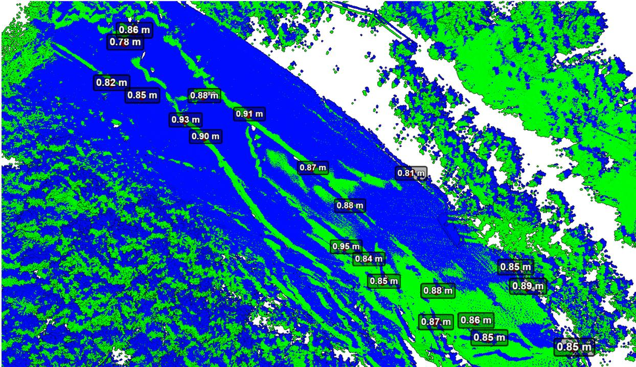
Figure 6: Distances found using manual extraction methods across the test site. Distances labeled are 3D distances and were transformed into 2D distances for use in this experiment.
