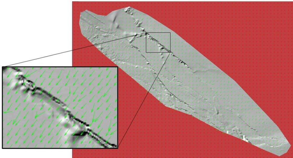
**Figure 7: Plot showing the displacement vectors from using the PIV algorithm on two hillshade rasters at the site overlaid on one of the hillshades. Vectors (green arrows) are drawn to scale.**
