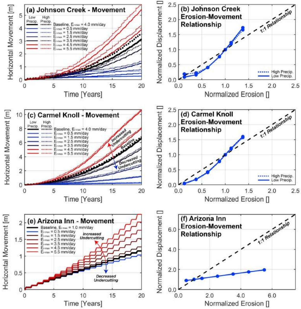
**Figure 1: Modeled landslide movements for 3 different landslide over the next 20 years for varying baseline erosion scenarios. Taken from Leshchinsky et al, 2019.**
