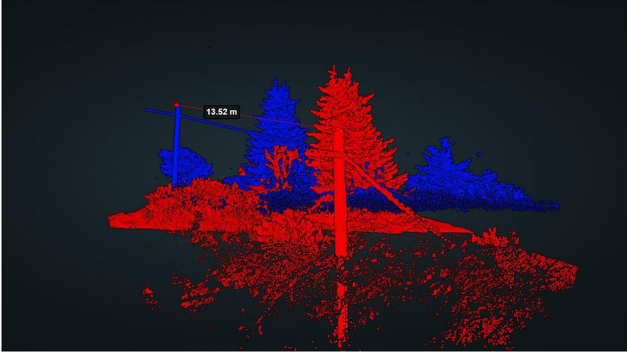
Figure 5: Example of manual measurement of a displaced object between two point clouds derived from different lidar survey epochs (before and after landslide failure).
