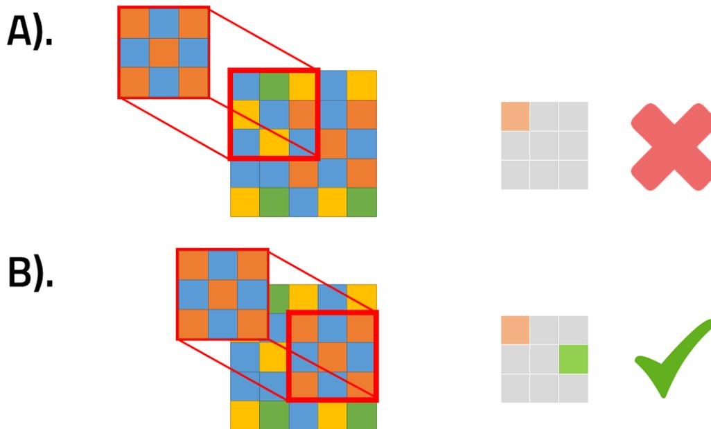
**Figure 2: Visual illustration of the 2D image cross correlation process. Each color represents a unique pixel value. In example A the window does not match the window of raster two so it calculates a low correlation value. In Example B the window does match the window of raster two, so it calculates a high correlation value, this would be perceived as a match.**
