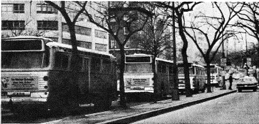
Multiple use of a near-side bus stop. Buses have completed loading and are leaving on green signal.
