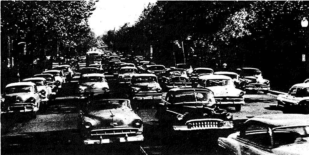
Four-lane urban arterial flow is provided here by prohibiting parking on one side during peak travel times.
