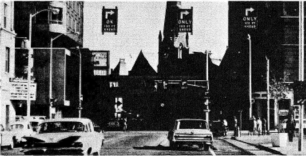
One-way urban arterial street in downtown area, showing signalized intersection with pavement laning.
