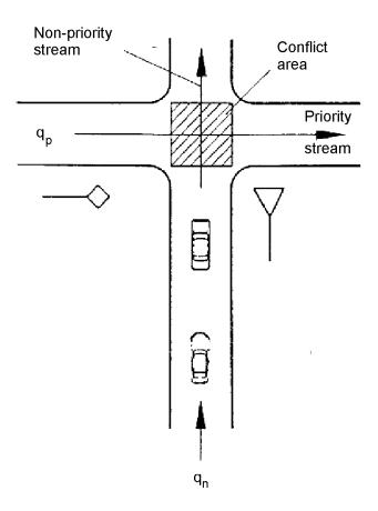
Figure 8.7 Illustration of the Basic Queuing System.
