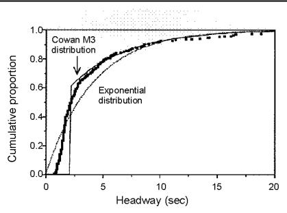
Figure 8.5 Arterial Road Data and a Cowan (1975) Dichotomized Headway Distribution (Higher flows example).
