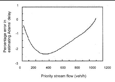
Figure 8.21 Percentage Error in Estimating Adams' Delay Against the Major Stream Flow for a Modified Single Lane Model (Troutbeck 1991).
