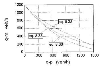
*Note:* Comparison of capacities for different types of headway distributions in the main street traffic flow for  $t_c = 6$  seconds and  $t_f = 3$  seconds. For this example,  $t_m$  has been set to 2 seconds.
