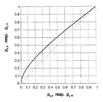
Figure 8.23 Reduction Factor to Account for the Statistical Dependence Between Streams of Ranks 2 and 3.
