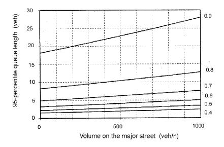
The parameter of the curves (indicated on the right side) is the degree of saturation (x).
