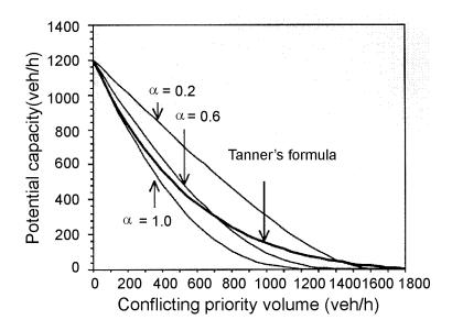
Figure 8.10 The Effect of Changing  $\alpha$  in Equation 8.31 and Tanner's Equation 8.36.
