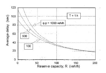
Figure 8.19 Average Delay, D, in Relation to Reserve Capacity R.
