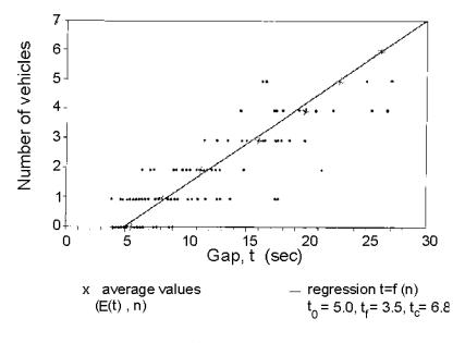
Figure 8.1 Data Used to Evaluate Critical Gaps and Move-Up Times (Brilon and Grossmann 1991).
