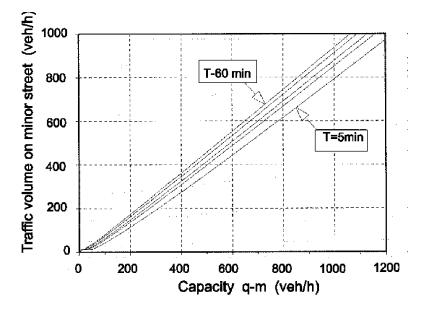
*Note:* The curves are given for time intervals T of 5, 10, 15, 30, and 60 minutes. Steady state conditions can be assumed if  $q_n$  is below the curve for the corresponding T-value.
