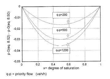
Figure 8.11 Probability of an Empty Queue: Comparison of Equations 8.50 and 8.52.
