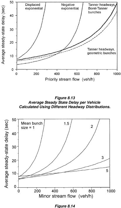
Average Steady State Delay per Vehicle by Geometric Platoon Size Distribution and Different Mean Platoon Sizes.
