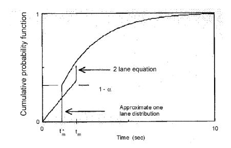
Figure 8.20 Modified 'Single Lane' Distribution of Headways (Troutbeck 1991).
