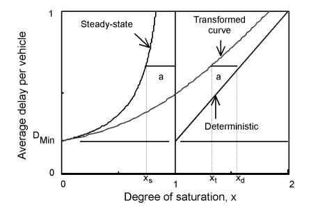
Figure 8.17 The Co-ordinate Transform Technique.
