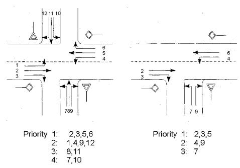
*Note:* The numbers beside the arrows indicate the enumeration of streams given by the Highway Capacity Manual (1994, Chapter 10).
