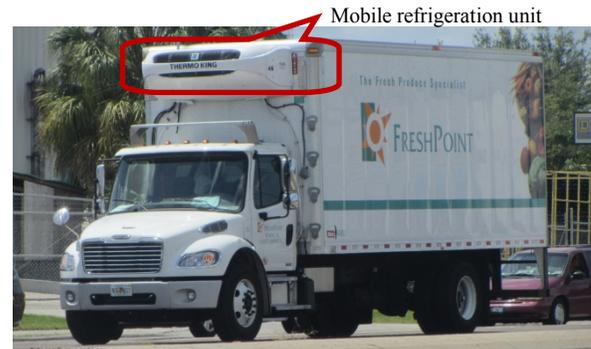
Figure 1. A typical produce delivery truck with MRU
