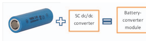
Figure 2. A single battery cell and a SC converter formed power module
