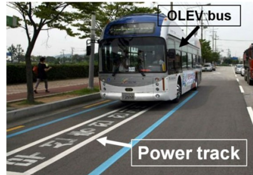
Figure 1. Implementation of OLEV system in Korea from [2].
