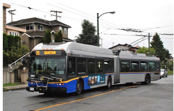
Figure 2. Catenary powered trolleybus in Vancouver from [14].
