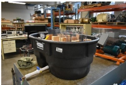
(a) Experimental flow tank set up.
