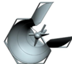
Fig. 1: Ducted turbine for hydrokinetic power generation. Adapted from [4].
