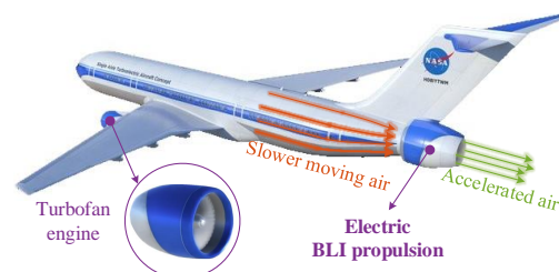
Fig. 3: STARC-ABL aircraft designed by NASA with a rear-mounted boundary layer ingesting fan [67].
