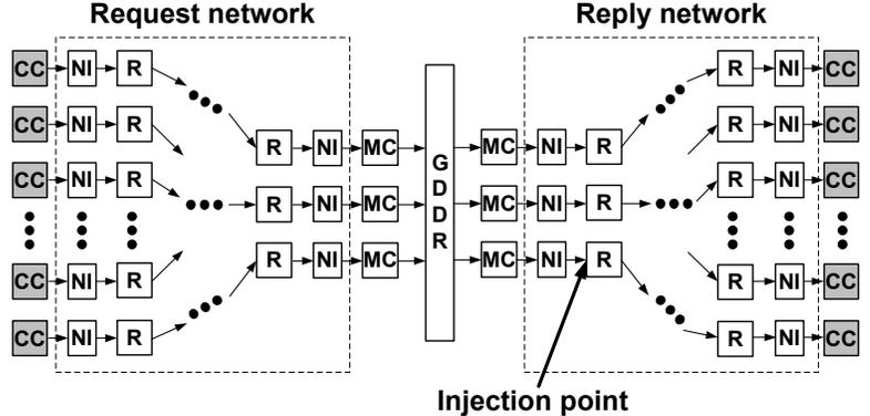
Figure 2: End-to-end traffic flow (CCs on both sides are the same).
