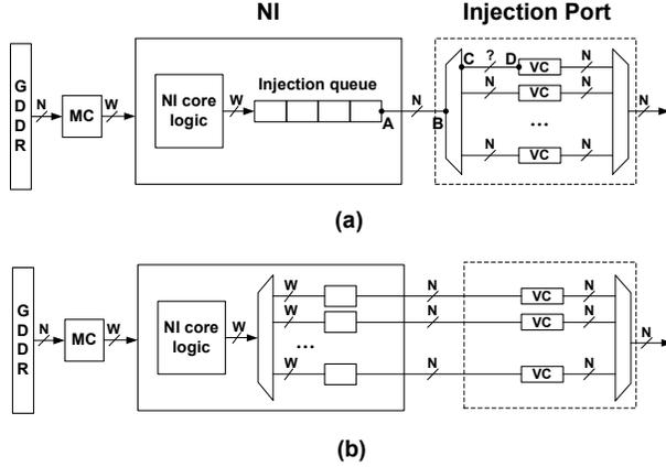
Figure 7: NI architecture: (a) enhanced baseline; (b) proposed.
