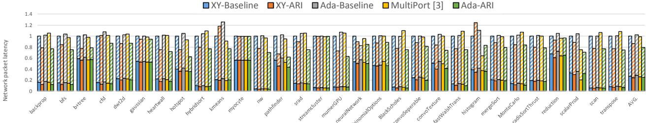
Figure 13: Average packet latency (striped: request packet latency; solid: reply packet latency).
