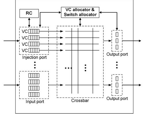
Figure 8: Injection port crossbar speedup.
