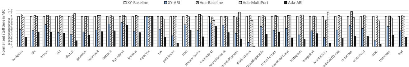
Figure 12: Data stall time in memory controllers due to NI injection queue full.
