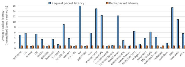
Figure 3: Request vs. reply packet latency.
