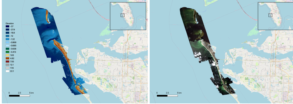
Figure 2: (Left) Bathymetry grid derived from bathymetric lidar data collected by NOAA’s CHARTS system in November, 2010. Data were resampled to align with AVIRIS pixels. (Right) True color composite (bands: R=29,G=20,B=12) of median pixel values from 3 overlapping AVIRIS scenes collected August 29th, 30th, and 31st of 2010.
