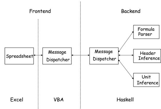
Figure 6. System architecture.
