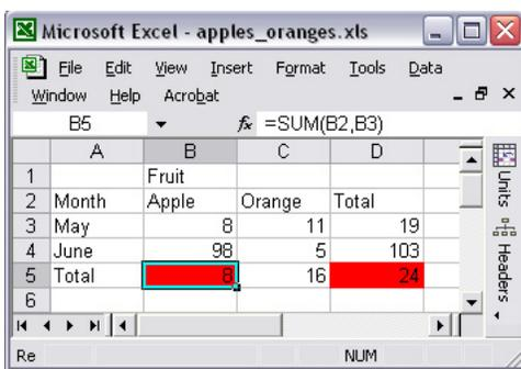
Figure 2. Identified range error.
