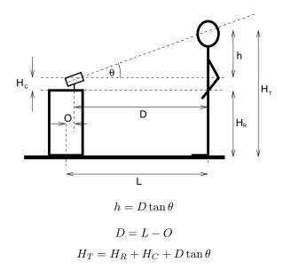
Figure 3: Calculating heights and distances using the laser range-finder.
