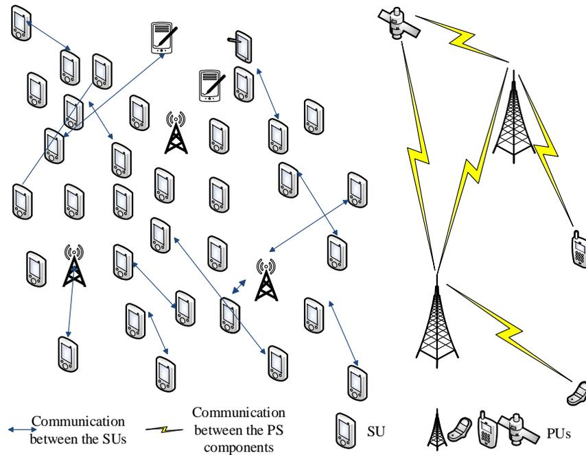
**Fig. 1.** Large scale DSA system.
