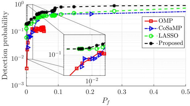
Fig. 8. Probability of detection as a function of the probability of false alarm with number of measurements  $m = 27$  and sensing SNR = 33 dB.
