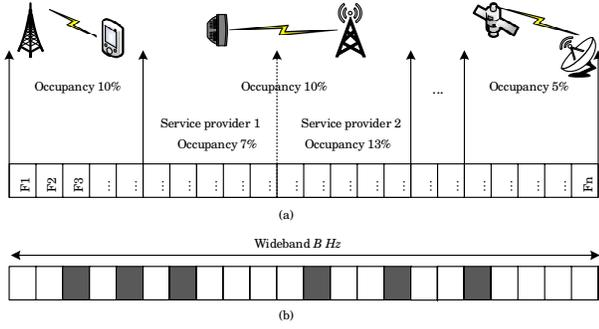
Fig. 1.  $n$  frequency bands occupied by heterogeneous applications with different occupancy rates. The grey bands are occupied by primary users while the white bands are vacant. (a) is the statistical allocation while (b) is a realization of allocation in a given region at a given time slot.
