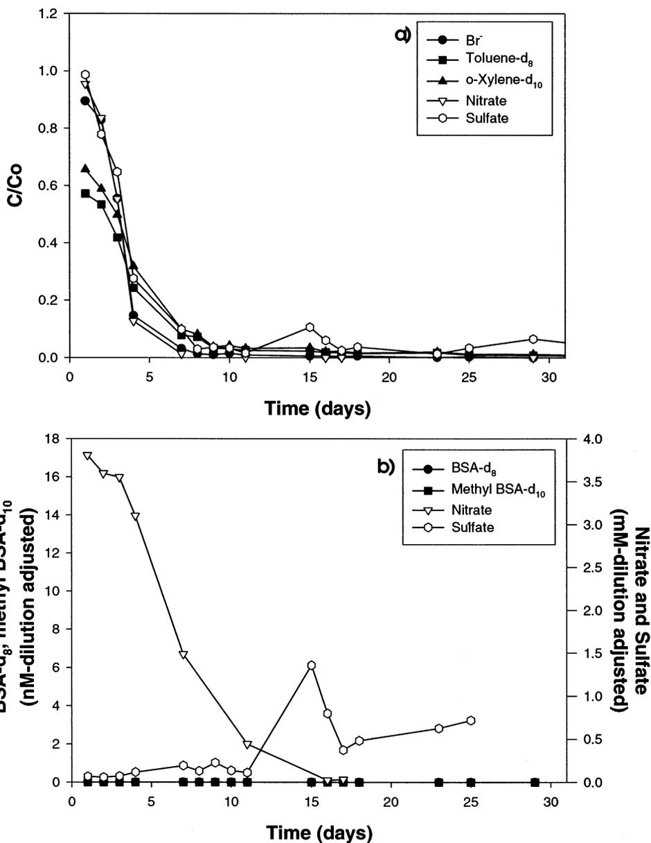
FIGURE 3. Extraction-phase breakthrough curve (a) for test in well CR12 at the Northwest Terminal site indicating dilution of injected toluene- $d_8$  and  $o$ -xylene- $d_{10}$  and (b) utilization of injected nitrate. Neither BSA- $d_8$  nor  $o$ -methyl-BSA- $d_{10}$  was detected.
