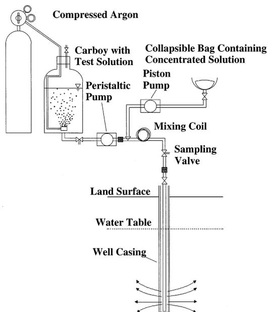
**FIGURE 1. Schematic of equipment used in single-well push–pull field tests.**
