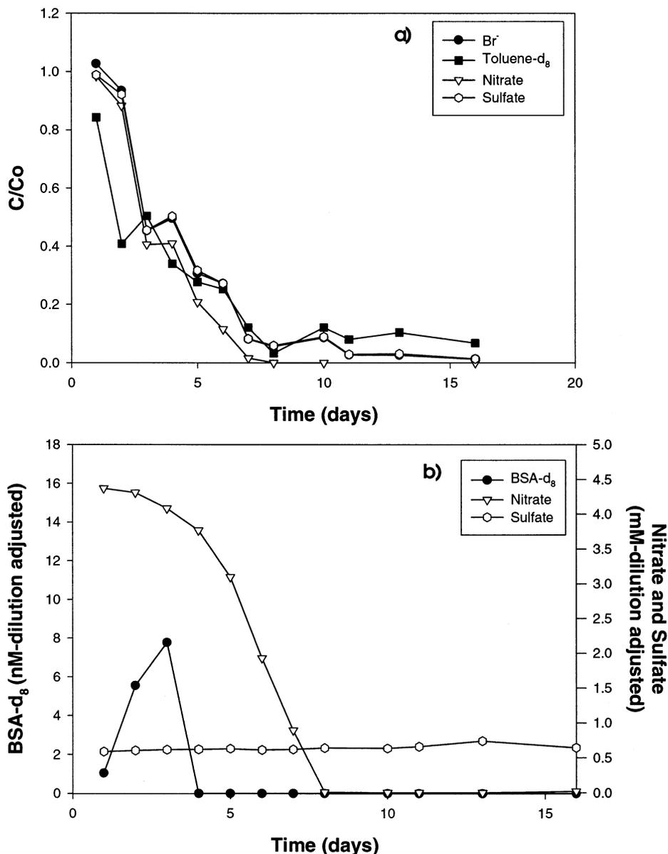
FIGURE 4. Extraction-phase breakthrough curve (a) for test in well 106s at the Kansas City site indicating dilution of injected toluene- $d_8$  and (b) utilization of injected nitrate and concurrent formation of BSA- $d_8$ . No *o*-methyl-BSA was expected because *o*-xylene- $d_{10}$  was not injected into this well.
