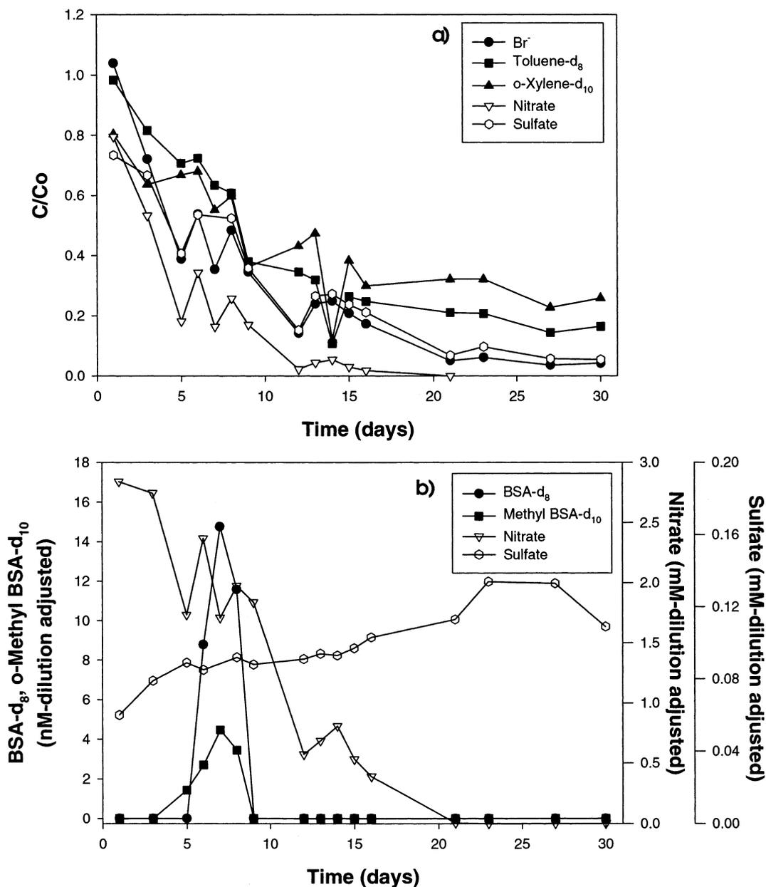
FIGURE 2. Extraction-phase breakthrough curve (a) for test in well CR15 at the Northwest Terminal site indicating dilution of injected toluene-*d*<sub>8</sub> and *o*-xylene-*d*<sub>10</sub> and (b) utilization of injected nitrate and concurrent formation of BSA-*d*<sub>8</sub> and *o*-methyl-BSA-*d*<sub>10</sub>.
