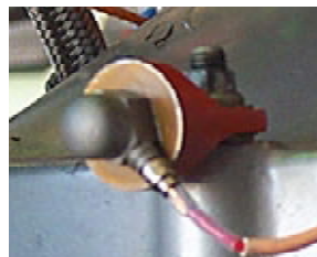
Figure 2. Accelerometer Mounting Bracket
