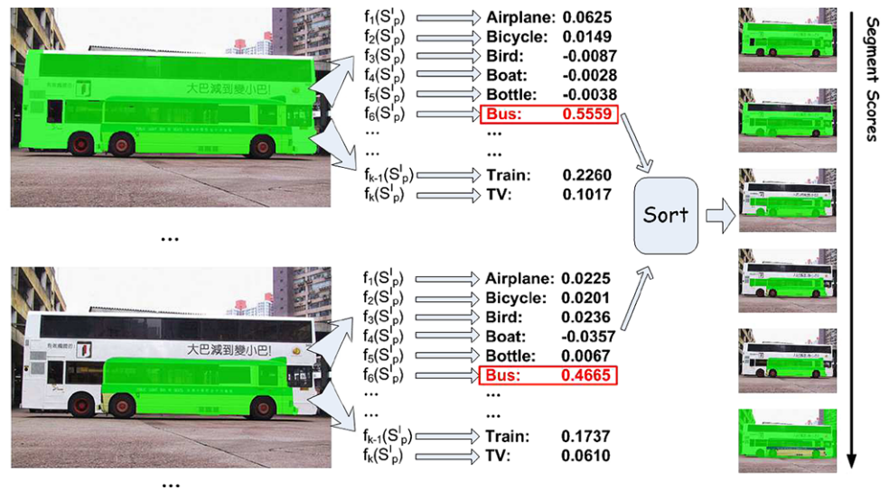
Fig. 4 An illustration of our segment categorization process. Each segment is given as input to regressors specialized for each category, producing estimated qualities. The maximal quality across categories is used to sort segments and decide on their category
