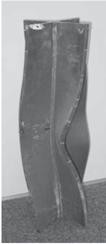
Figure 5.26 Column Tested to Failure through Local Buckling Photo courtesy Perry Green
