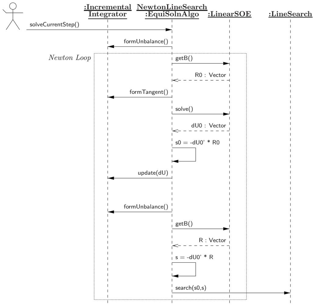
**Fig. 14.** Sequence diagram for one time step using the Newton–Raphson algorithm with line search
