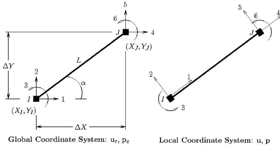
Fig. 1. Element degrees of freedom in the global and local coordinate systems
