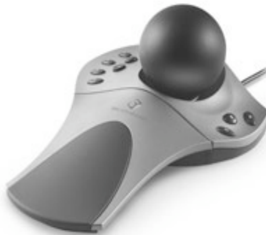
Figure 7.3: a 6DF device, the SpaceBall 5000 from Connexion Systems (permission not yet granted)
