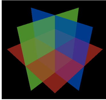
Figure 5.21: the partially transparent planes broken into quadrants and drawn back-to-front
