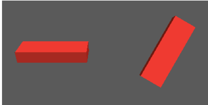
Figure 2.14: the results from two different orderings of the same rotations
