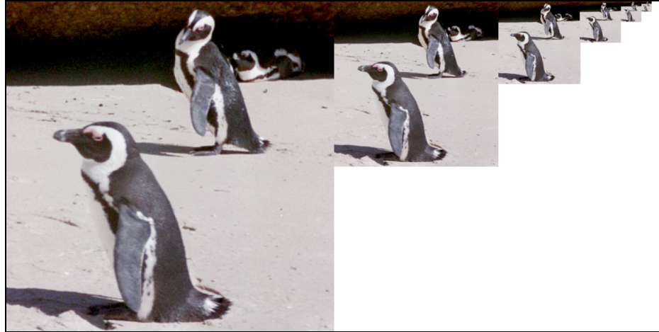
Figure 8.8: a texture map holding several versions of a base texture for MIP mapping
