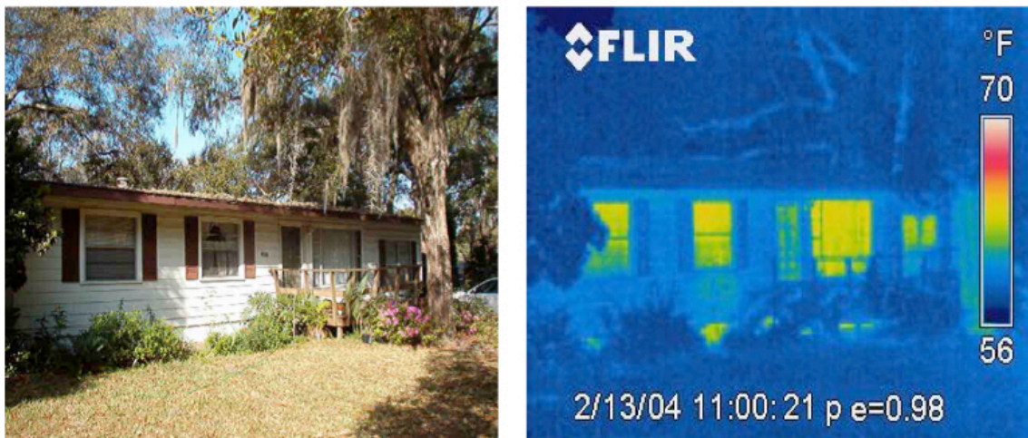
Figure 5.14: A house shown in a normal photograph (left) and with thermal imaging (right); from [MCC]
