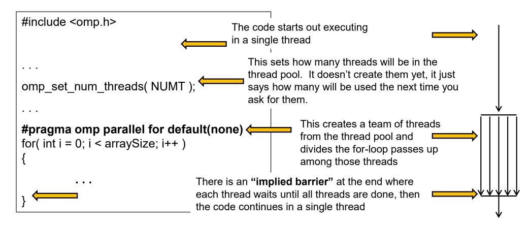
This tells the compiler to parallelize the for-loop into multiple threads. Each thread automatically gets its own personal copy of the variable *i* because it is defined within the for-loop body.
