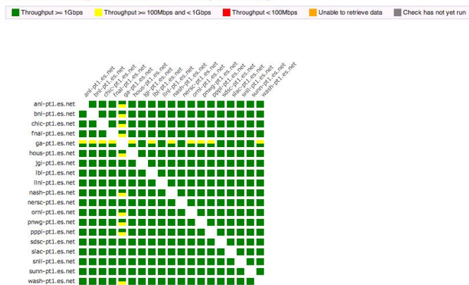
Figure 2: Regular perfSONAR monitoring of the ESnet infrastructure. The color scales denote the “degree” of throughput for the data path. Each square is halved to show the traffic rate in each direction between test hosts.
