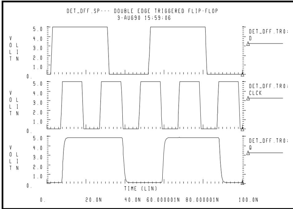
Figure 22-13: Double Edge Triggered Flip-Flop Response
