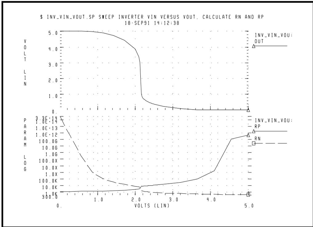
**Figure 22-17: RP and RN as a Function of VIN**
