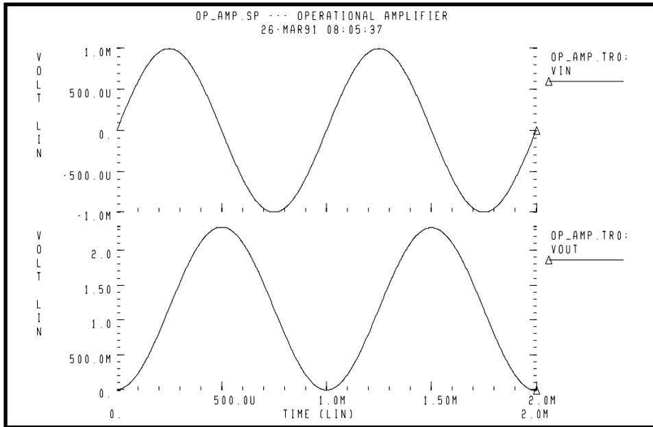
Figure 22-33: Transient Analysis Response<sup>1</sup>.
