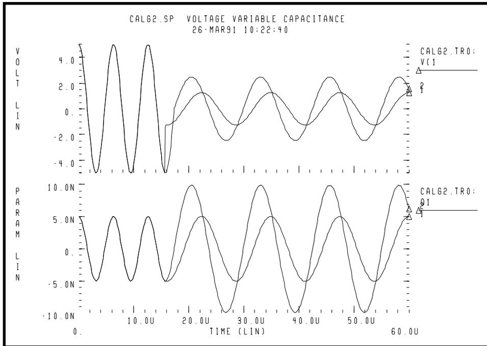
**Figure 22-37: Correct Result Corresponding to CTYPE=1**
