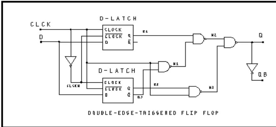
Figure 22-12: Double Edge Triggered Flip-Flop Schematic
