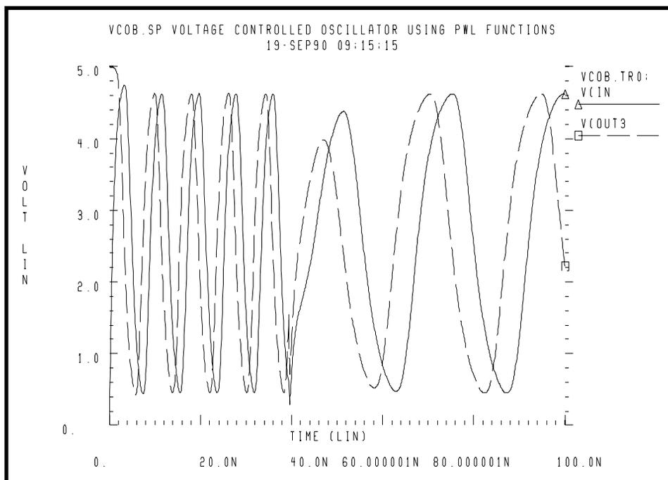
**Figure 22-36: Voltage Controlled Oscillator Response**
