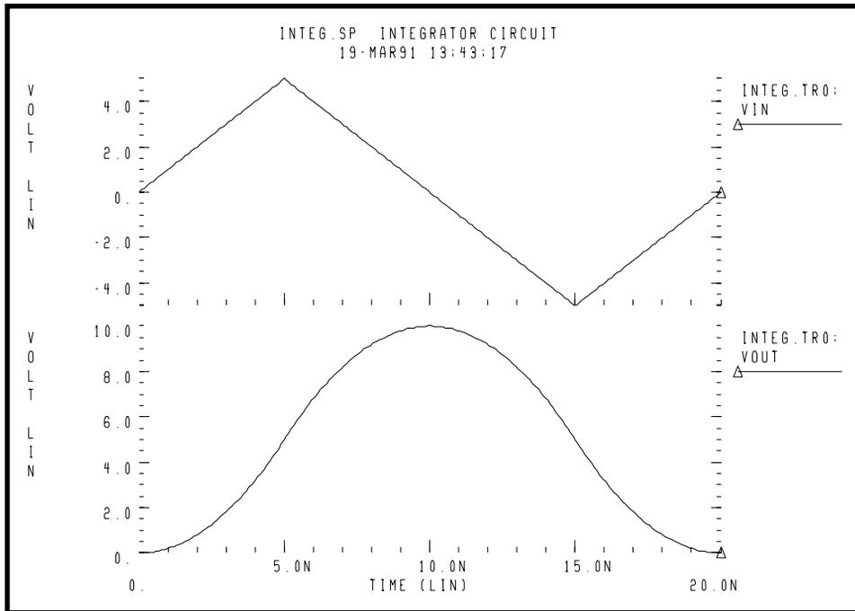
**Figure 22-22: Response of Integrator to a Triangle Waveform**
