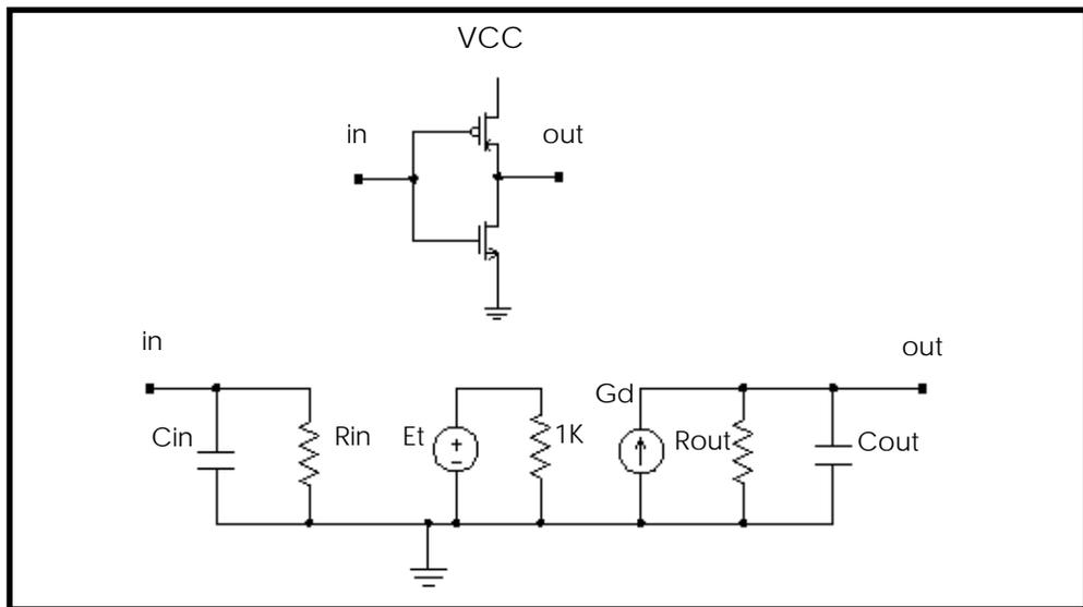
**Figure 22-18: CMOS Inverter and its Equivalent Circuit**
