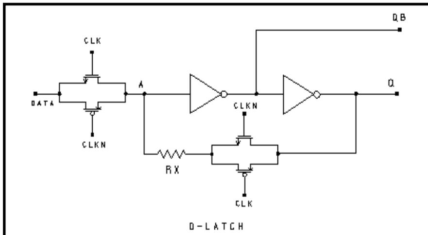
Figure 22-10: D-Latch Circuit
