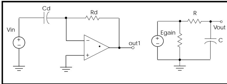
**Figure 22-23: Differentiator Circuit**
