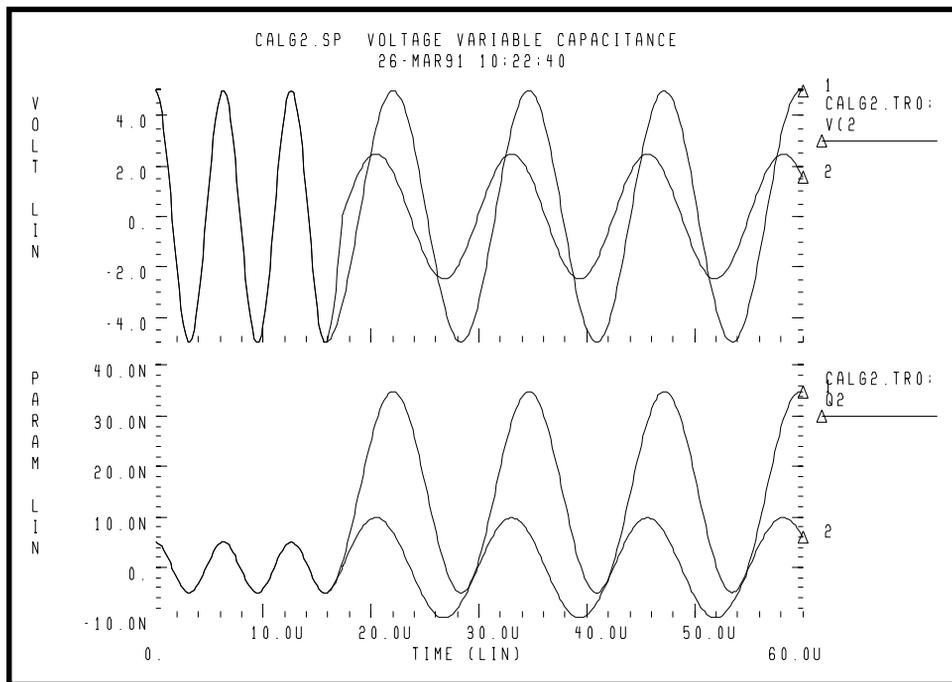
**Figure 22-38: Incorrect Result Corresponding to CTYPE=0**
