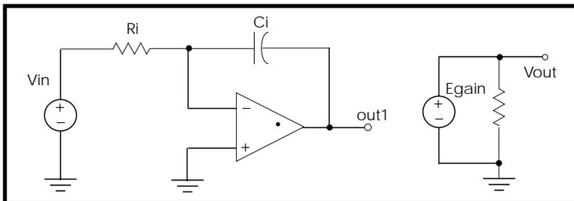
**Figure 22-21: Integrator Circuit**
