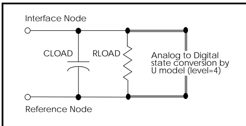
**Figure 22-6: – Analog to Digital Converter Element**
