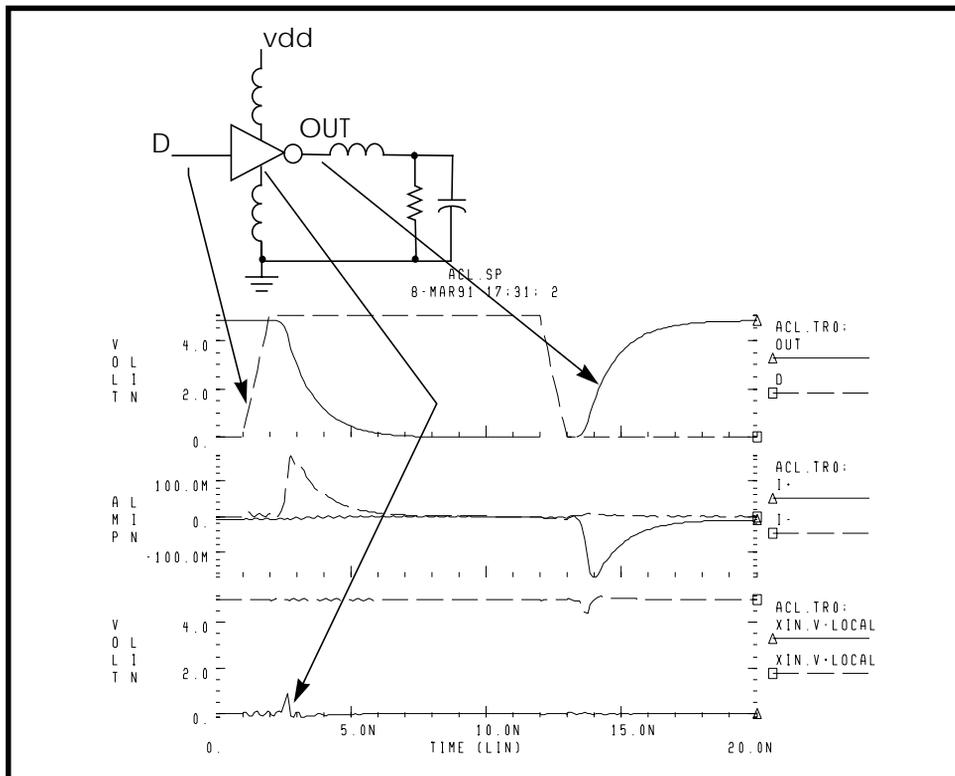
**Figure 22-14: ACL Family Output Buffer**
