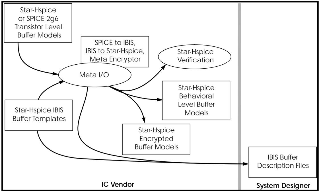
**Figure 23-1: IC Vendor Design Data Flow Using Meta I/O**
