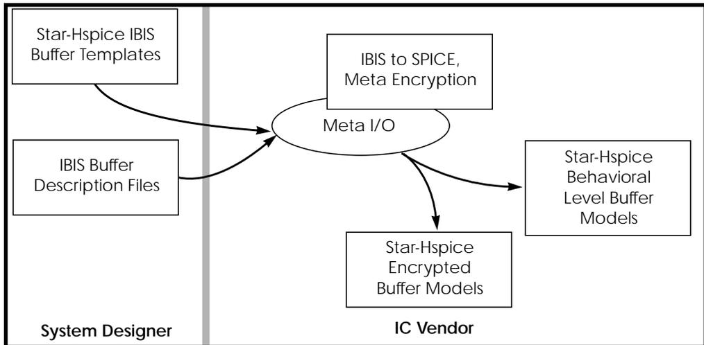
**Figure 23-2: – System Design Data Flow Using Meta I/O**
