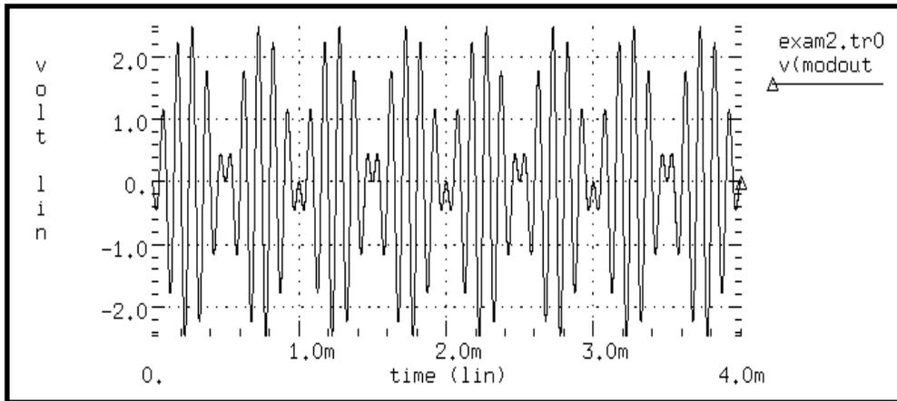
**Figure 25-7: Modulated Signal**
