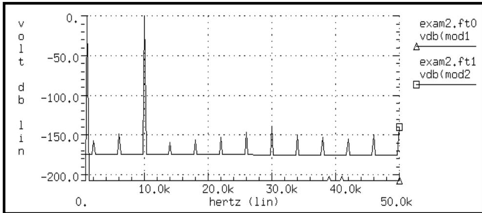
**Figure 25-10: Modulating and Modulated Signal Spectrum**
