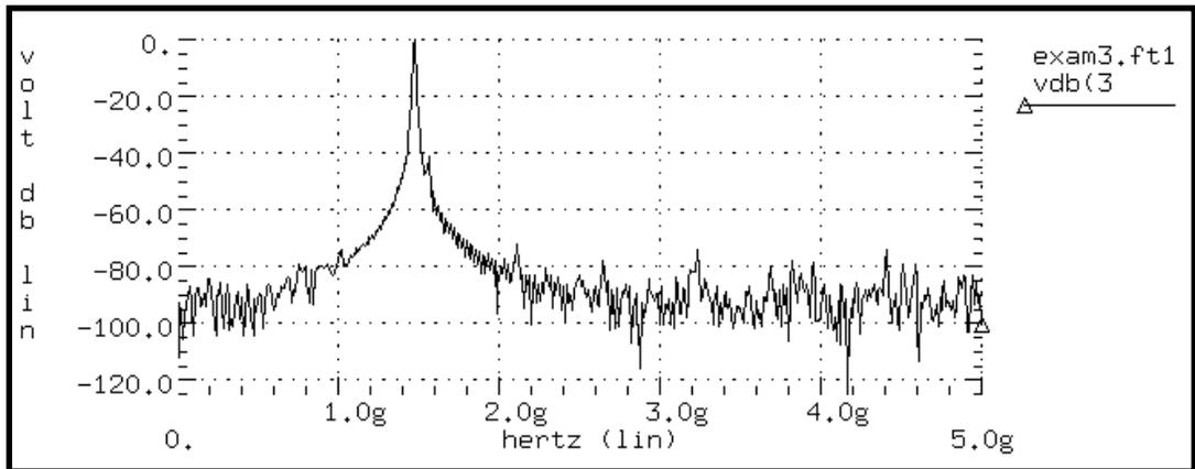
**Figure 25-16: Mixer Output Spectrum, Bartlett Window**
