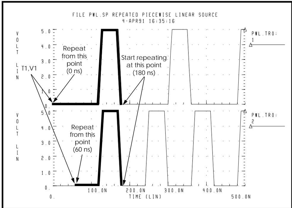
**Figure 5-4: Results of Using the Repeat Function**
