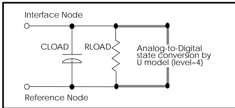
**Figure 5-8: Analog-to-Digital Converter Element**
