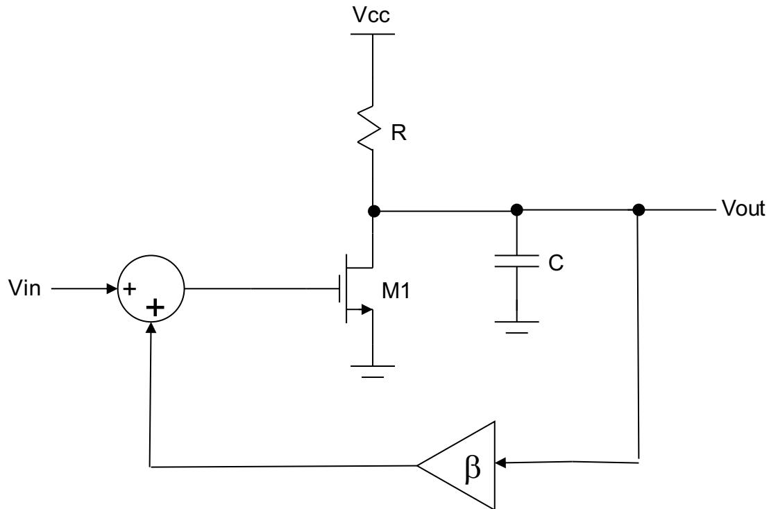
**Prob-6** For the circuit shown below, find (a) minimum gain  $k$  if  $R=1K\Omega$  and (b) minimum value of  $R$  if  $k=0.25$  for which the circuit will oscillate and determine the expression for frequency of oscillation in both the cases. Consider  $ro=\infty$  and  $gm=1m A/V$  for all the PMOS.
