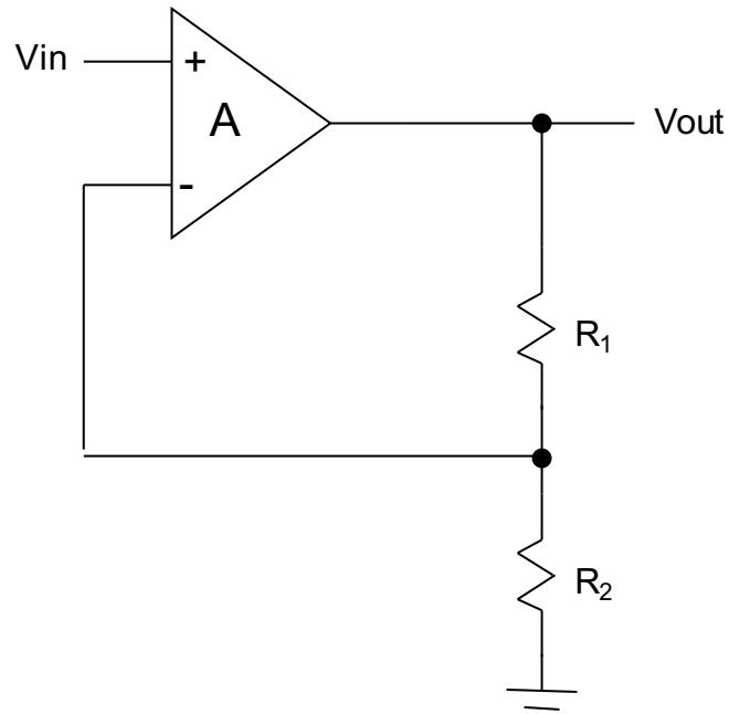
**Prob-4.** A system is said to be unstable if any of the poles lie in right half of the s-plane. This property can be used to convert a second order system into oscillator by using negative feedback and choosing a proper feedback function. Find the closed loop transfer function  $V_{out}(s)/V_{in}(s)$  of the system and show how the location of poles change w.r.t  $k$  in s-plane.
