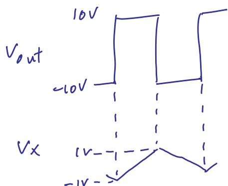
$$I = C \frac{dV}{dt} \rightarrow \text{slope} = \frac{\Delta V}{\Delta t} = \frac{I}{C} = \frac{10}{RC} = \frac{10}{(50k\Omega)(25pF)}$$
