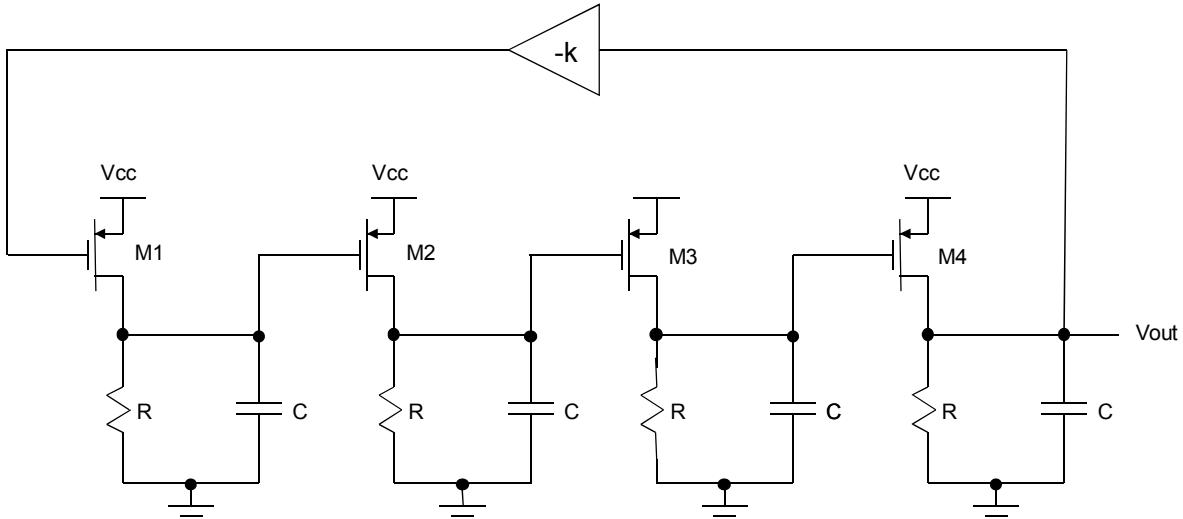
Each stage to contribute  $45^\circ$  phase delay  $\rightarrow$  results in positive FB loop.
