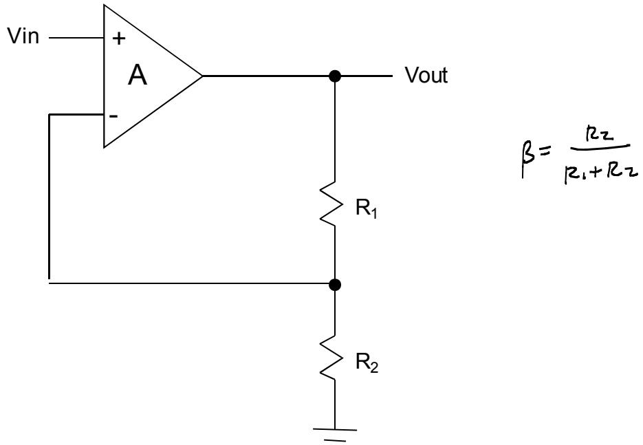
$$\text{Closed loop gain} = \frac{V_{out}}{V_{in}} = \frac{A}{1 + A\beta} = \underbrace{\frac{1}{\beta}}_{\substack{\text{ideal} \\ \text{gain}}} \frac{A\beta}{1 + A\beta}$$
