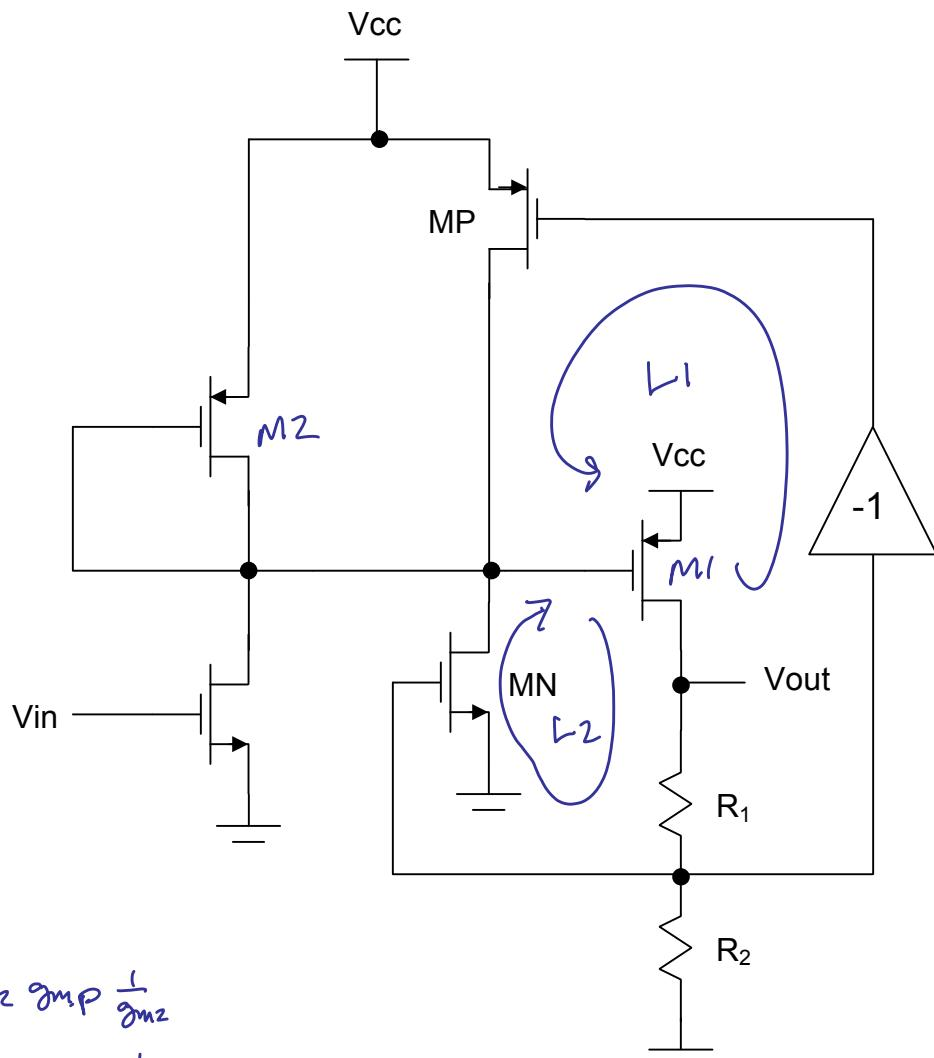
$$L_1 = -g_{m1} R_2 g_{mp} \frac{1}{g_{m2}}$$
