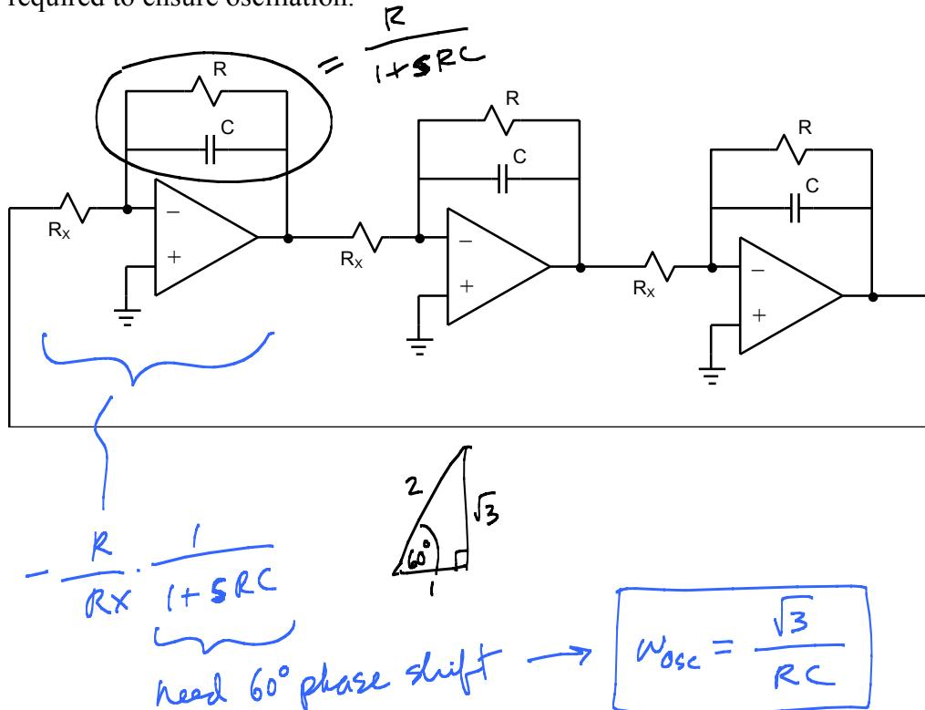
$$\left| \text{Loop gain} (s = j\omega_{\text{osc}}) \right| = \left( \frac{R}{R_x} \frac{1}{2} \right)^3 \geq 1 \quad \text{to ensure oscillation}$$
