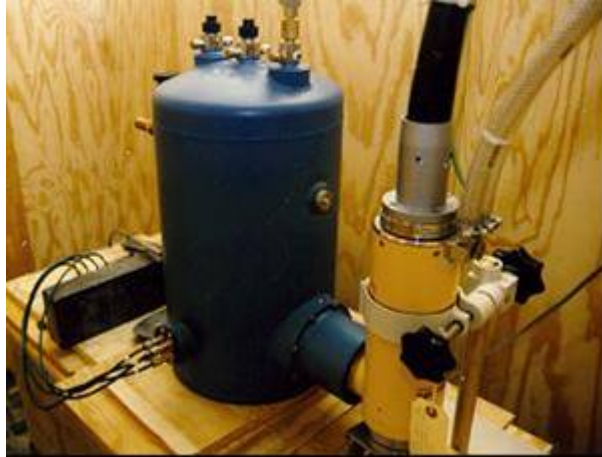
Figure 3.1. LEXR source in test chamber.
