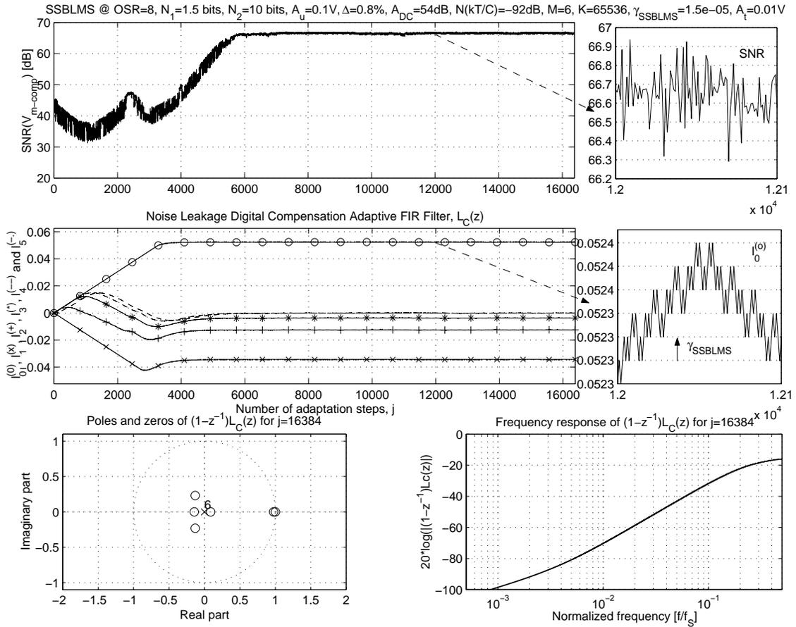
Figure 4.10: Adaptive compensation process (differentiated  $v_q[n]$ )
