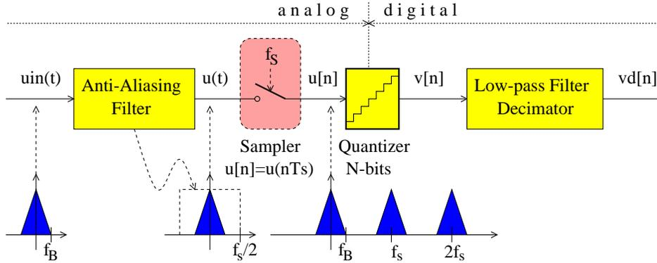
Figure 2.6: General oversampling analog-to-digital converter ( $OSR = 2$ )
