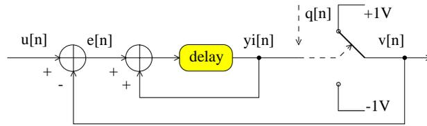
Figure 2.12: Time-domain model of the first-order delta-sigma ADC
