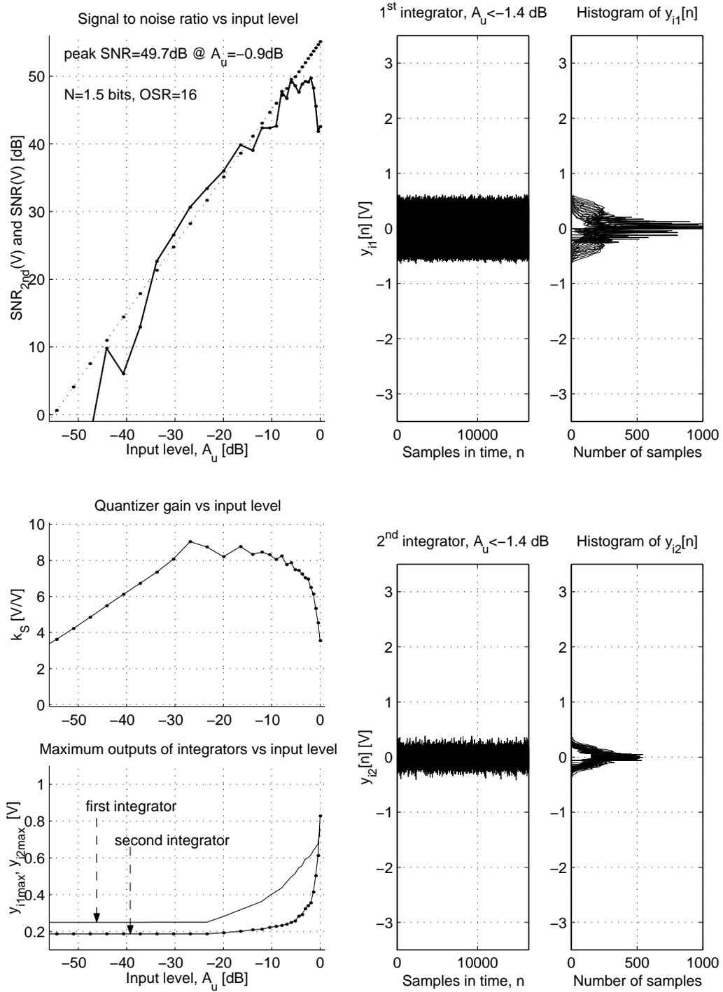
Figure 2.28: Internal voltage swings for  $a_1 = \frac{1}{4}$ ,  $a_2 = \frac{1}{2}$ ,  $b_1 = 1$ ,  $b_2 = \frac{1}{2}$ ,  $k = 8$
