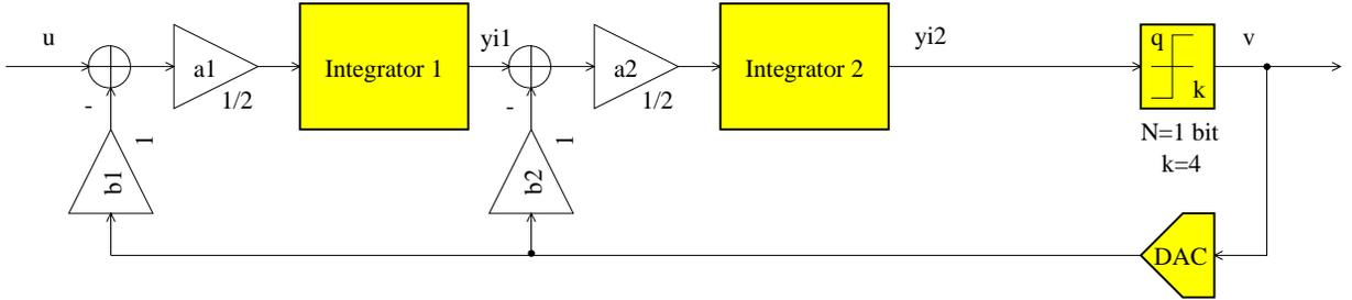
Figure 2.14: Second-order single-bit delta-sigma ADC
