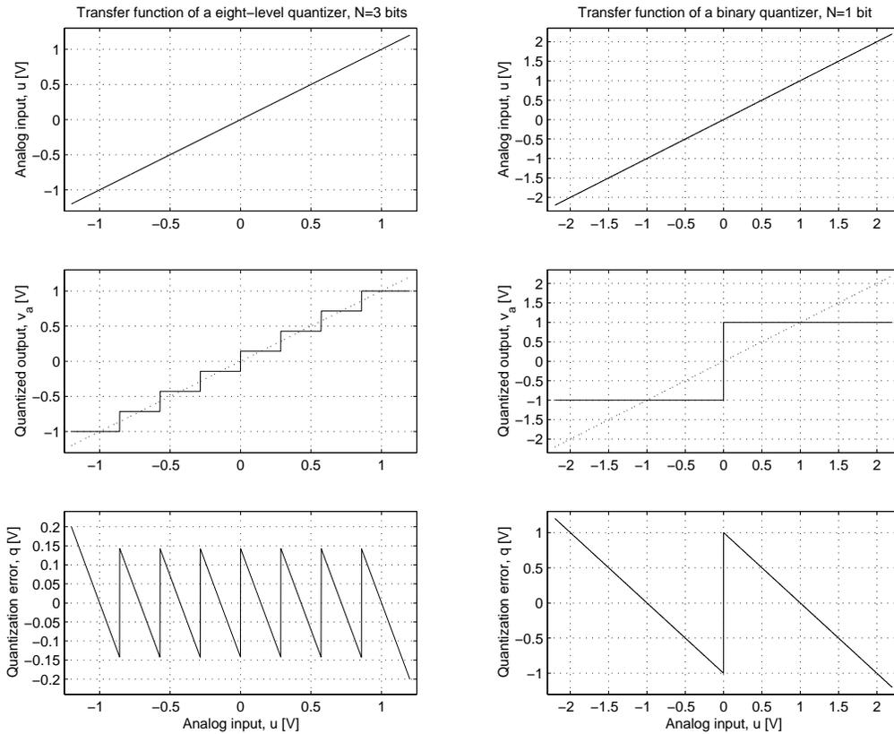
Figure 2.3: Transfer function of an ideal  $N$ -bit quantizer for (a)  $N = 3$  bits and (b)  $N = 1$  bit
