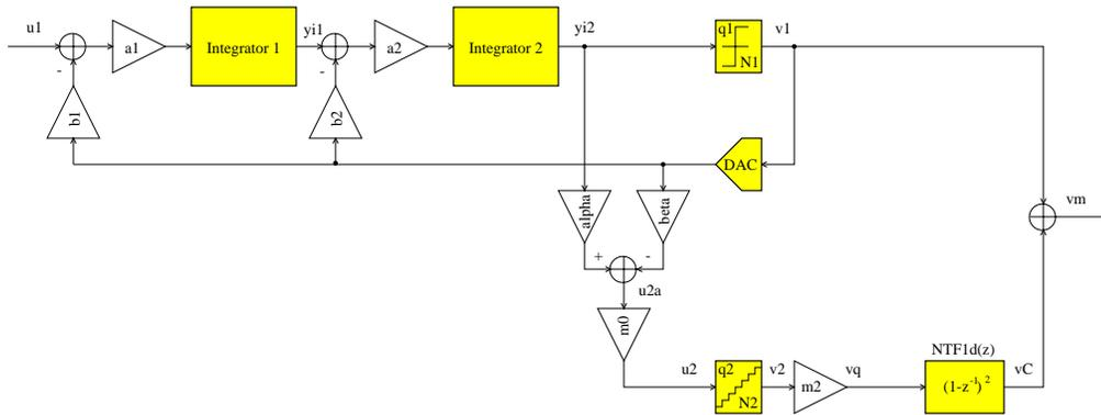
Figure 3.3: Improved standard structure of the cascaded 2-0  $\Delta\Sigma$  ADC
