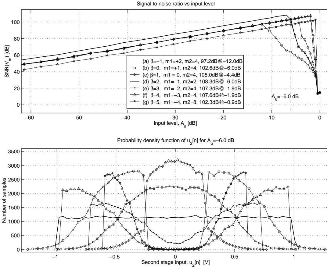
Figure 3.8:  $SNR$  performance and  $PDF(u_2[n])$  for different  $\beta$  and  $m_1$ , assuming ideal MASH,  $OSR = 16$ ,  $N_1 = 1$  bit and  $N_2 = 12$  bits
