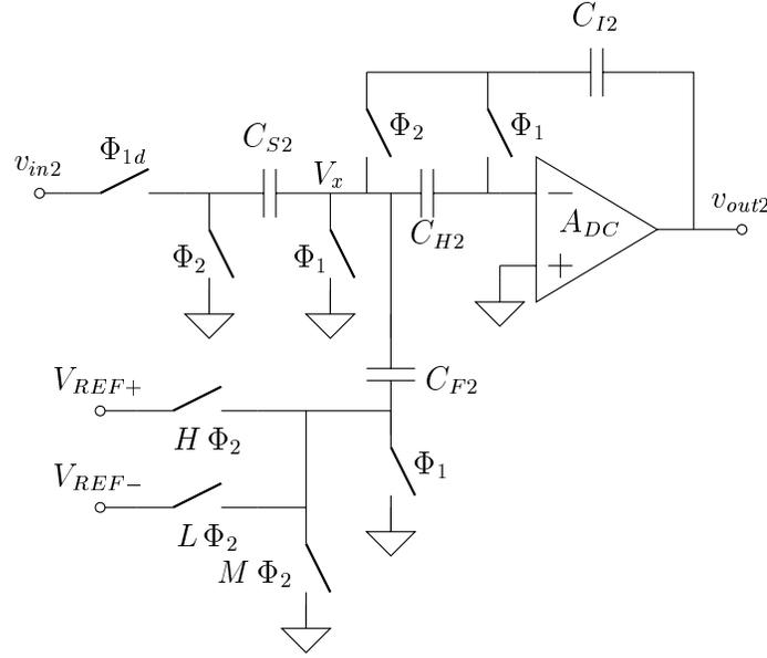
Figure 5.2: Second integrator from the first stage of the MASH ADC
