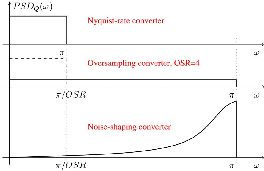
Figure 2.7: The power spectral density of the quantization noise  $PSD_Q(\omega)$  for different converters
