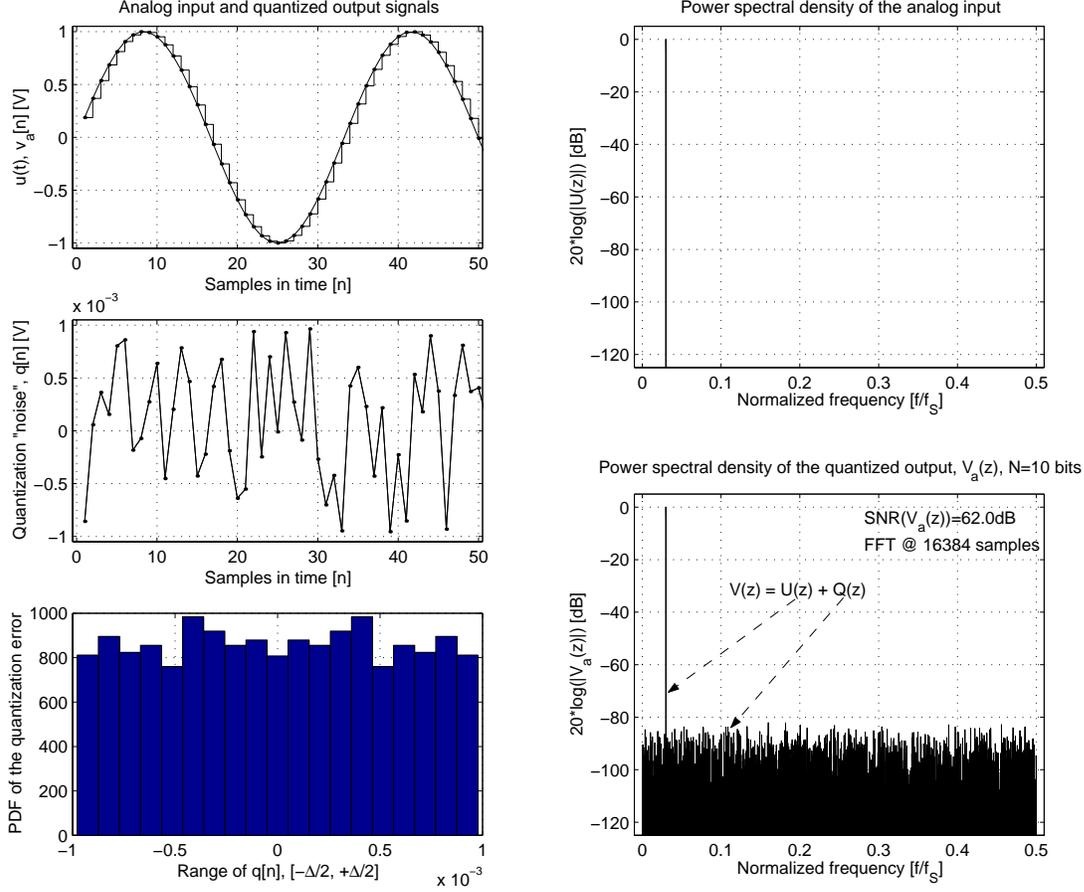
Figure 2.5: The spectrum of a quantized sinewave for  $N=10$  bits
