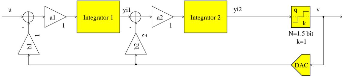
Figure 2.24: Second-order tri-level delta-sigma ADC
