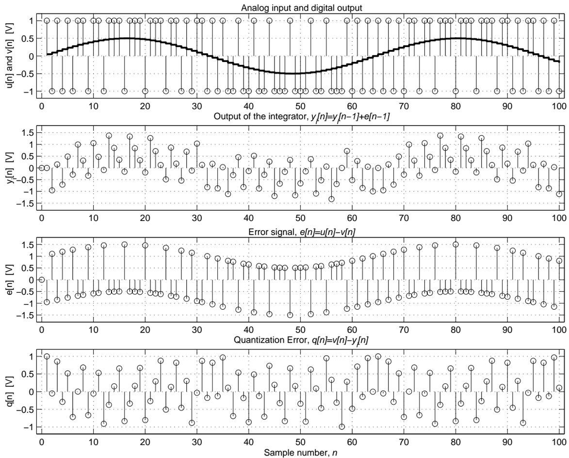
Figure 2.13: First-order delta-sigma ADC response in time to a half-scale in-band sinusewave input ( $OSR = 32$ )
