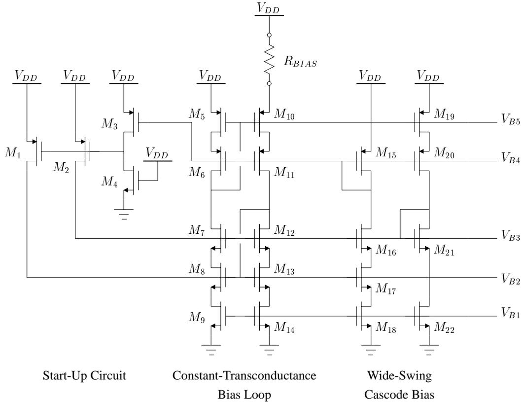
Figure 5.5: Generation of the bias voltages for the opamps
