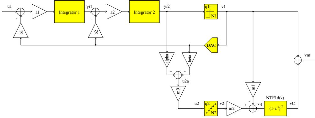
Figure 3.5: General structure of the cascaded 2-0 delta-sigma ADC
