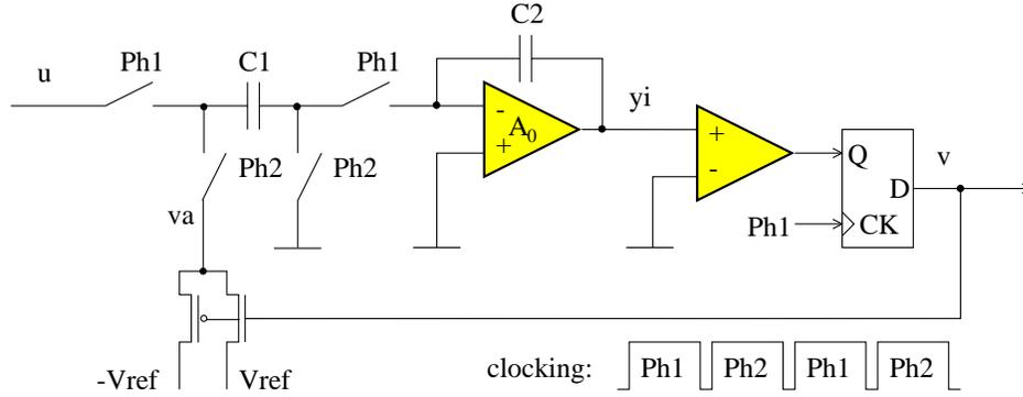
Figure 2.11: Switched-capacitor first-order delta-sigma ADC
