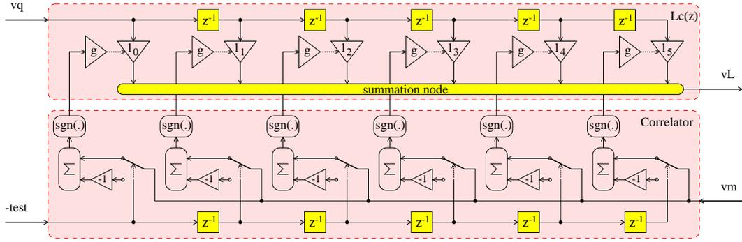
Figure 4.3: Simplified hardware implementation of the correlator using a binary test signal  $test[n]$  to update the coefficients  $l_i$  of the adaptive noise-leakage compensation digital filter  $L_C(z)$  ( $g = \gamma_{SSBLMS}$  and  $M - 1 = 5$ )
