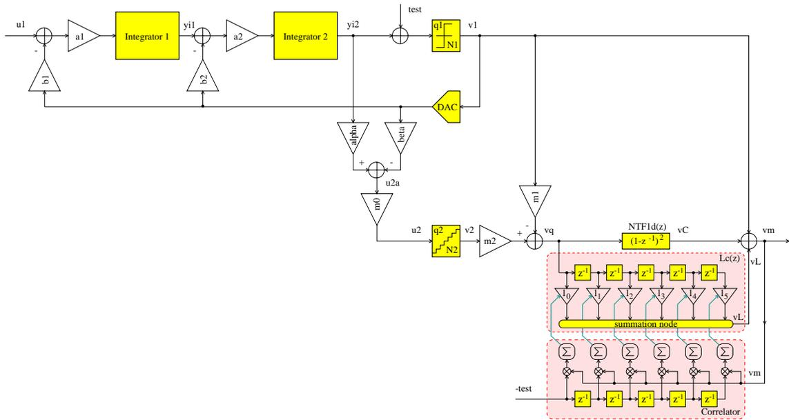
Figure 4.2: Adaptive digital noise-leakage compensation scheme using a test signal  $test[n]$  for the general cascaded 2-0 delta-sigma ADC ( $M = 6$ )
