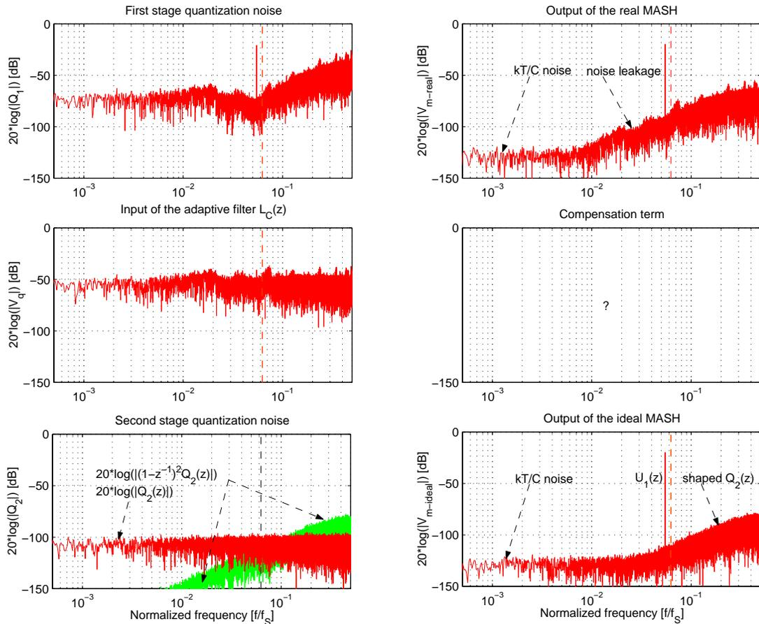
Figure 3.12: Noise leakage in the general cascaded 2-0 delta-sigma ADC ( $OSR = 8$ ,  $N_1 = 1.5$  bits,  $N_2 = 10$  bits,  $A_u = 0.1$  V,  $\Delta_C = 0.8\%$ ,  $A_{DC} = 54$  dB and  $N\left(\frac{kT}{C}\right) = -92$  dB)
