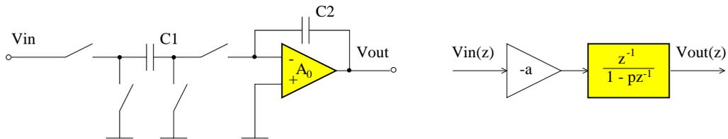
Figure 3.11: Switched-capacitor integrator and its linear model
