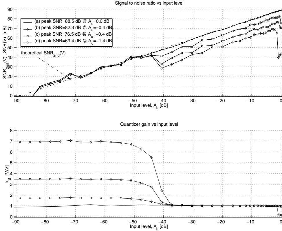
Figure 2.26: Second-order multibit (100 levels, gain  $k = 1$ ) delta-sigma ADC's  $SNR$  and quantizer gain curves for  $b_2 = 2a_1b_1$  and (a)  $\frac{1}{a_1a_2b_1} = 1$ , (b)  $\frac{1}{a_1a_2b_1} = 2$ , (c)  $\frac{1}{a_1a_2b_1} = 4$  and (d)  $\frac{1}{a_1a_2b_1} = 8$
