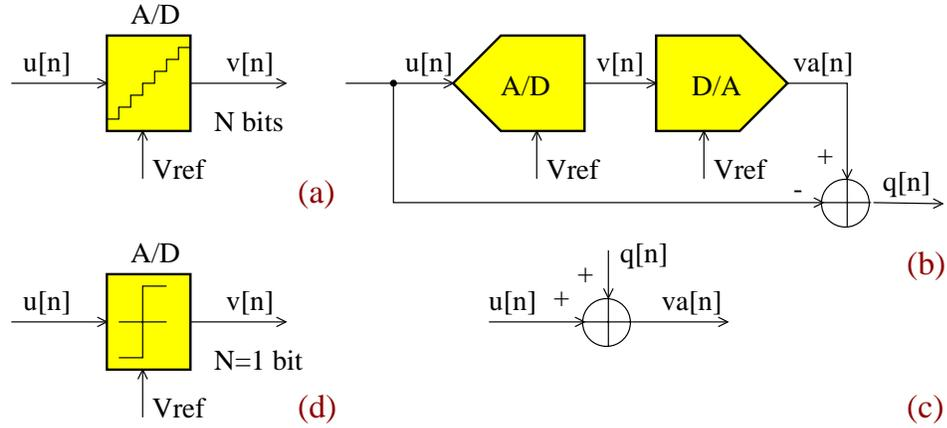
Figure 2.2: (a) Ideal  $N$ -bit quantizer; (b) quantization error generation:  $q[n] = v_a[n] - u[n]$ ; (c) discrete-time domain modeling of the quantization process:  $v_a[n] = u[n] + q[n]$ ; (d) ideal single-bit quantizer
