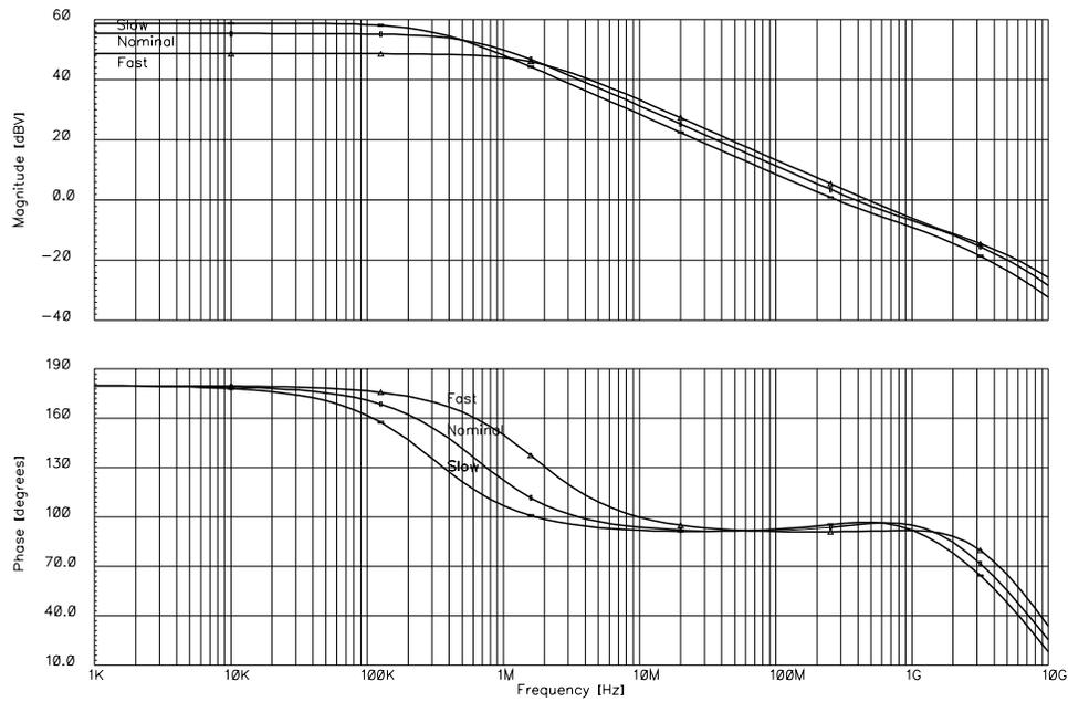
Figure 5.15: Operational amplifier frequency response
