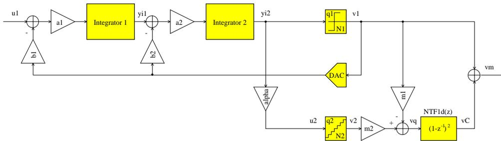
Figure 3.4: Simplified structure of the cascaded 2-0 delta-sigma ADC
