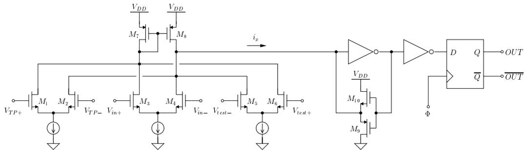
Figure 5.7: Comparator used in the tri-level quantizer
