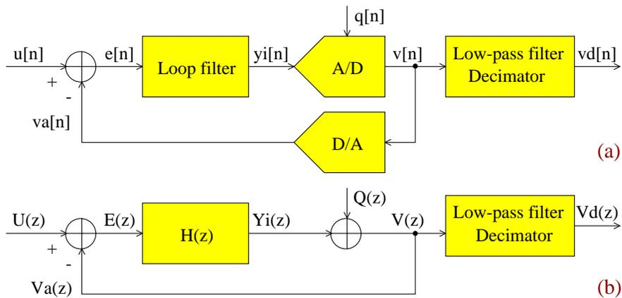
Figure 2.8: (a) General structure of a noise-shaping ADC and (b) its linearized model (for the DAC a unity gain was assumed)
