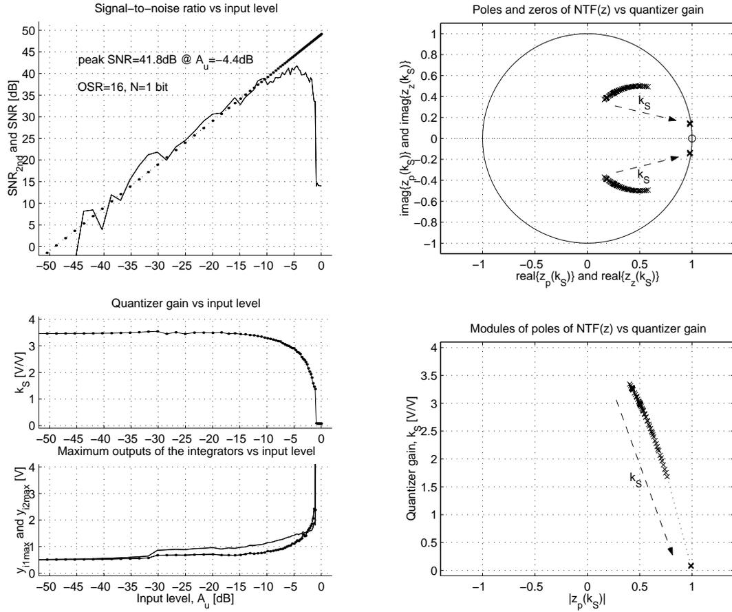
Figure 2.22: Stability analysis of the second-order delta-sigma ADC ( $a_1 = \frac{1}{2}$ ,  $a_2 = \frac{1}{2}$ ,  $b_1 = 1$ ,  $b_2 = 1$  and  $k = 4$ )
