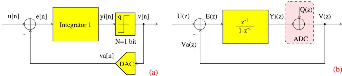
Figure 2.10: (a) First-order delta-sigma ADC and (b) its linearized model
