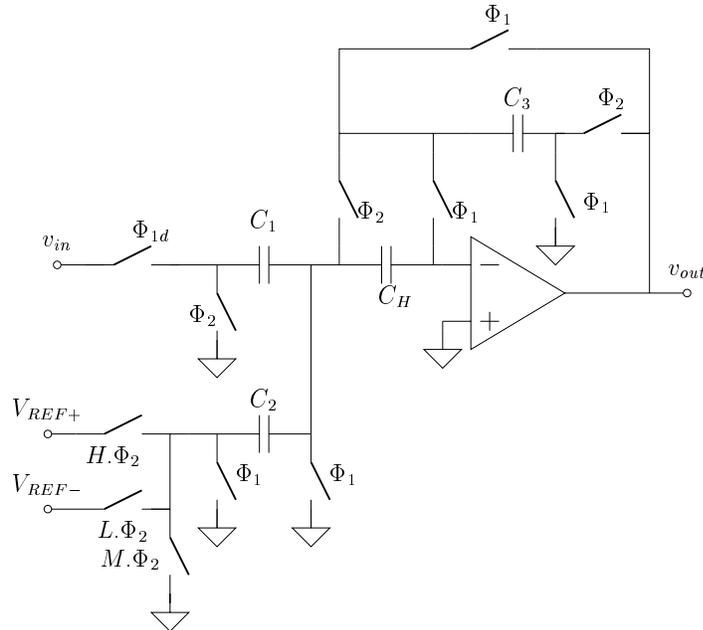
Figure 5.10: Analog subtraction circuit providing the second-stage input  $u_2$
