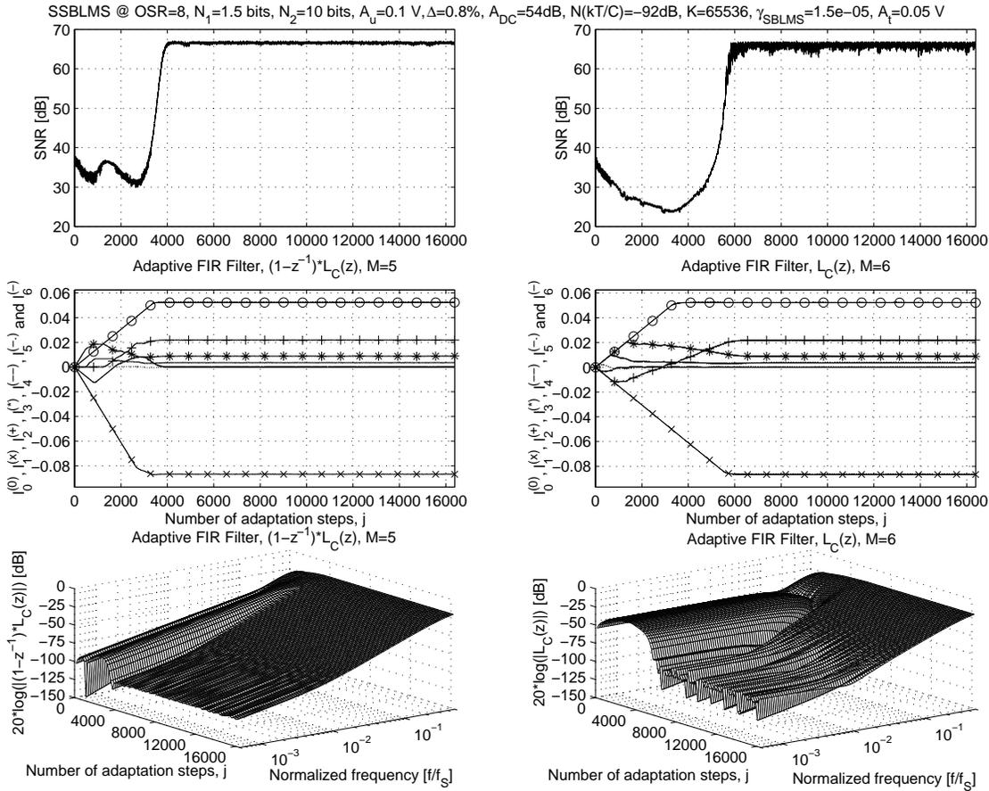
Figure 4.9: (a) Reducing the ripple of the adaptation noise using a differentiator,  $M = 6$ ; (b) adaptation process without differentiator,  $M = 7$
