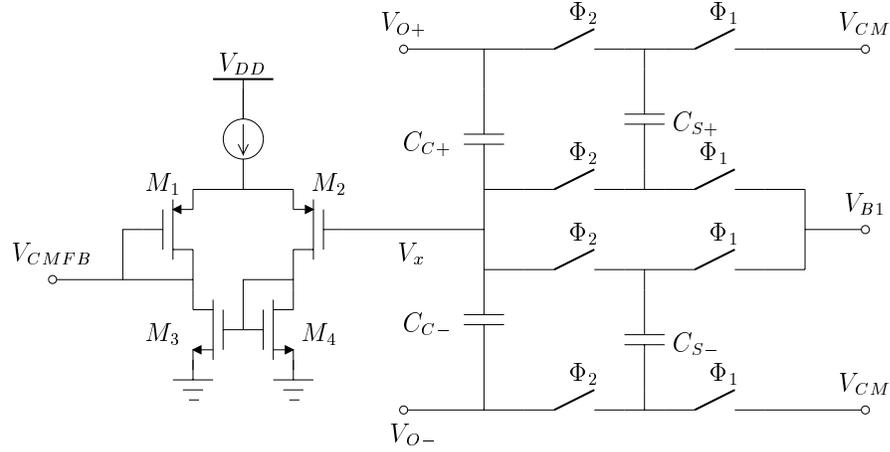
Figure 5.4: Common-mode feedback circuit for the opamps
