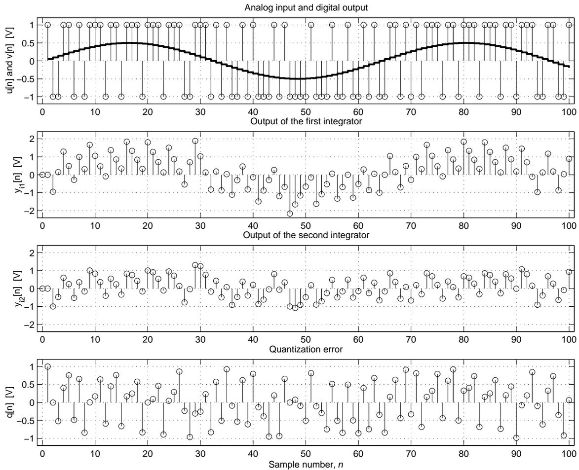
Figure 2.20: Second-order delta-sigma ADC response in time to a half-scale in-band sinewave input ( $a_1 = \frac{1}{2}$ ,  $a_2 = \frac{1}{2}$ ,  $b_1 = 1$ ,  $b_2 = 1$ )
