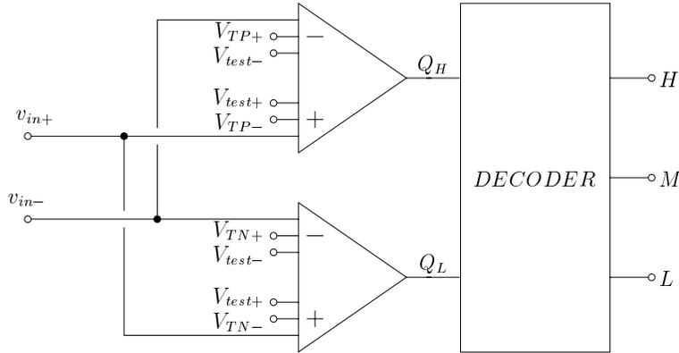
Figure 5.6: Tri-level quantizer for the first stage of the MASH ADC
