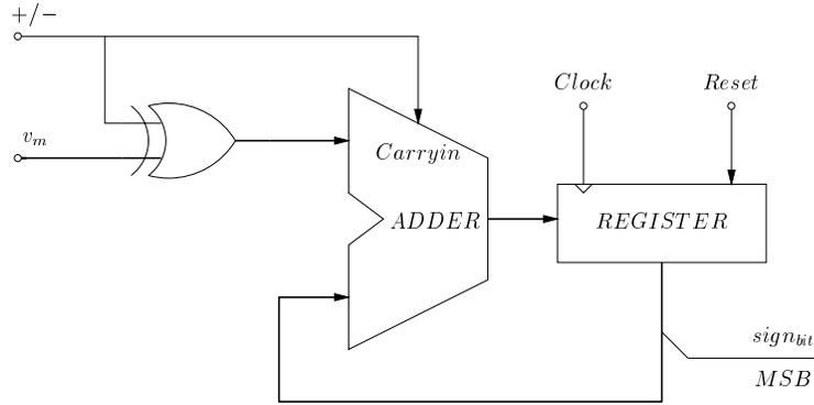
Figure 5.13: Accumulator for the adaptive filter
