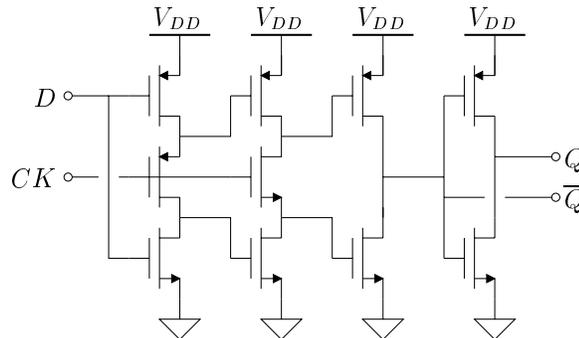
Figure 5.8: TSPC flip-flop used in the comparator
