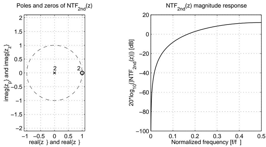
Figure 2.16: Noise transfer function of the second-order delta-sigma ADC
