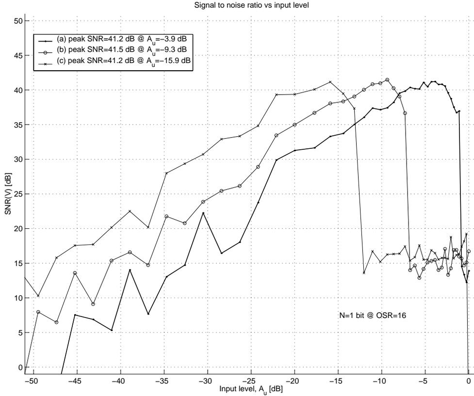
Figure 2.23:  $SNR$  performance of second-order single-bit delta-sigma ADCs for (a)  $|STF(z)| = 1$ ,  $a_1 = \frac{1}{2}$ ,  $a_2 = \frac{1}{2}$ ,  $b_1 = 1$ ,  $b_2 = 1$  [50], (b)  $|STF(z)| = 2$ ,  $a_1 = 1$ ,  $a_2 = 1$ ,  $b_1 = \frac{1}{2}$ ,  $b_2 = 1$  [52], (c)  $|STF(z)| = 4$ ,  $a_1 = 1$ ,  $a_2 = 1$ ,  $b_1 = \frac{1}{4}$ ,  $b_2 = \frac{1}{4}$ .
