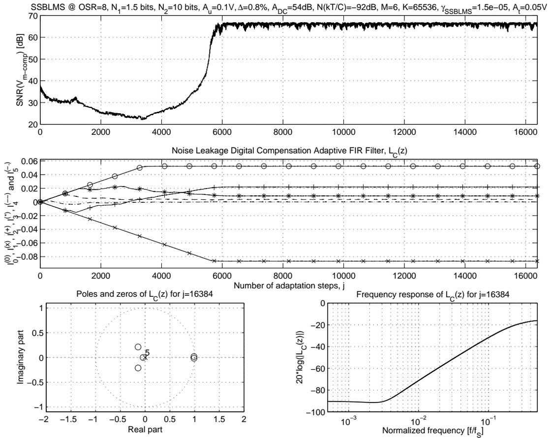
Figure 4.5: Adaptive compensation process ( $K = 2^{16}$ ,  $\gamma_{SSBLMS} = 1.5 \cdot 10^{-5}$ )
