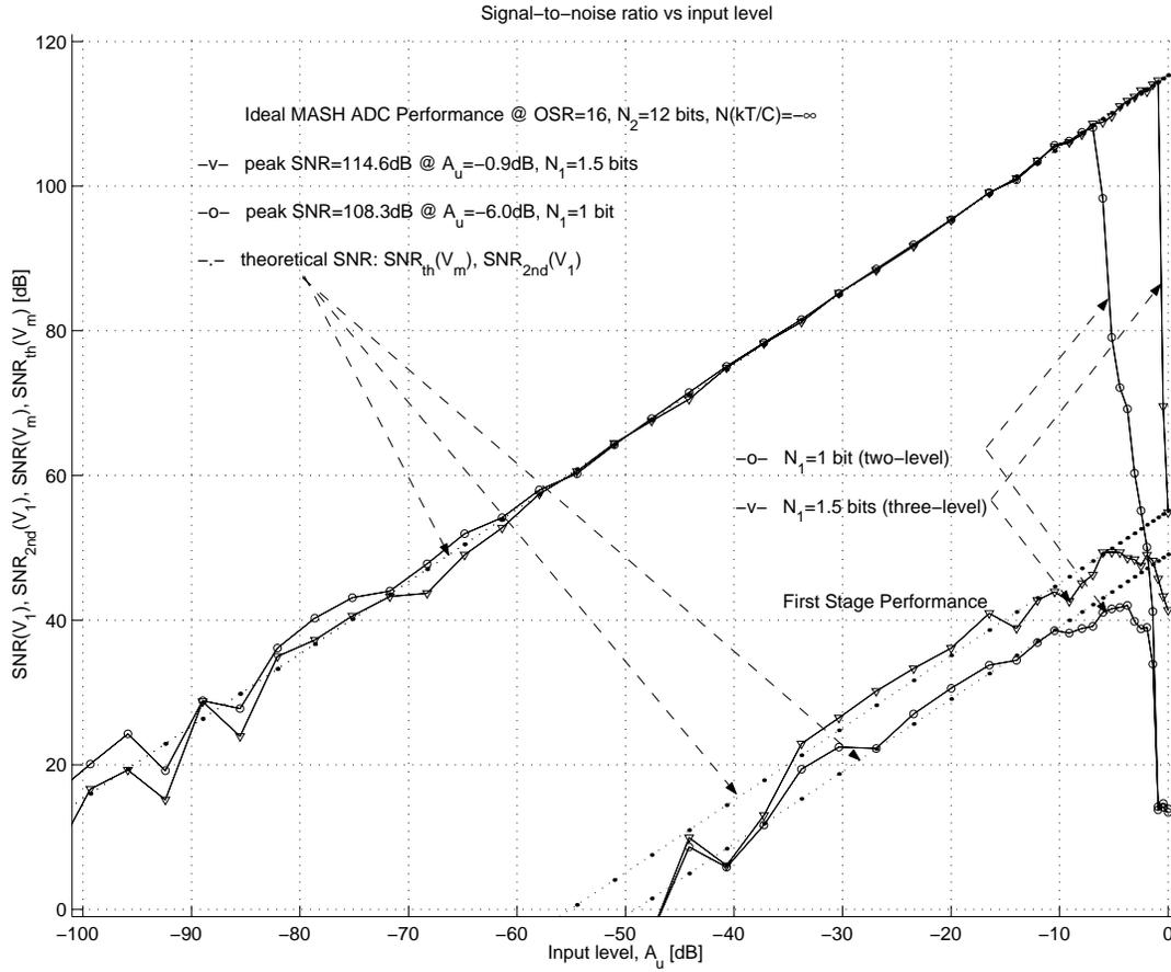
Figure 3.9: Comparative performance of the general MASH ( $\beta = 2$ ,  $m_1 = -1$ ,  $m_0 = \frac{1}{2}$ ,  $m_2 = 2$ ) for bi-level ( $N_1 = 1$  bit,  $k_1 = 1$ ) and tri-level ( $N_1 = 1.5$  bits,  $k_1 = 8$ ) first stage ( $a_1 = \frac{1}{4}$ ,  $a_2 = \frac{1}{2}$ ,  $b_1 = 1$ ,  $b_2 = \frac{1}{2}$ )
