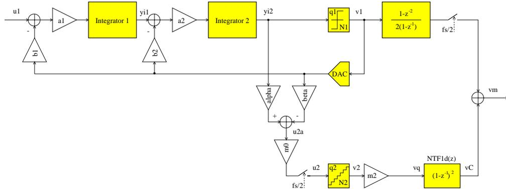
Figure 5.12: MASH structure with reduced sample-rate requirement for the second stage
