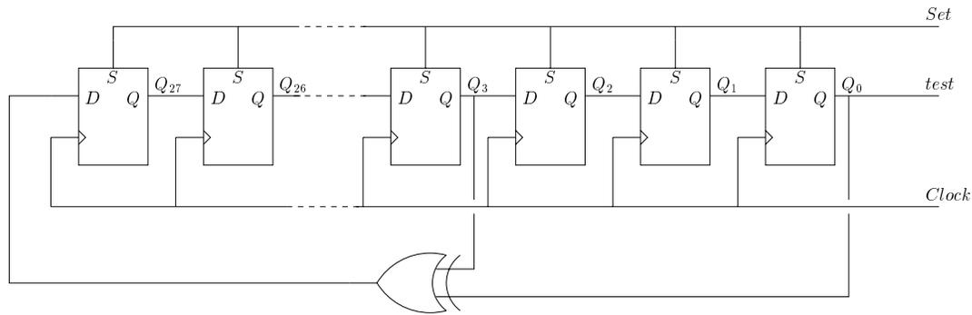
Figure 5.14: 28-bit maximum-length sequence generator
