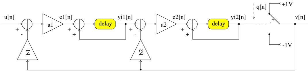
Figure 2.19: Time-domain model of the second-order delta-sigma ADC
