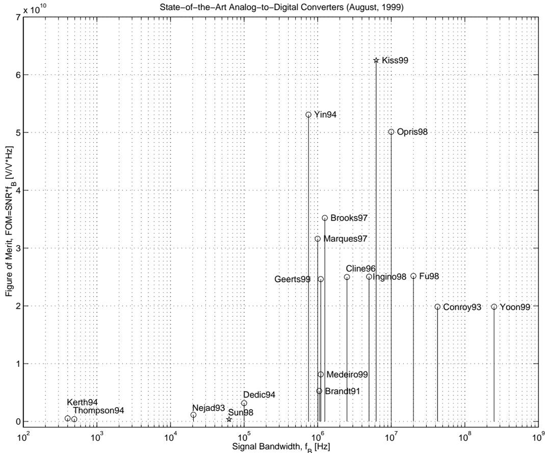
Figure 1.2: Figure of merit for state-of-the-art ADCs
