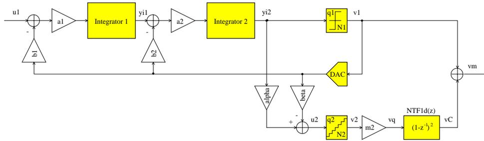
Figure 3.2: Standard structure of the cascaded 2-0 delta-sigma ADC
