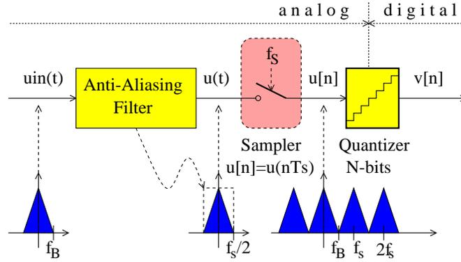
Figure 2.1: General analog-to-digital converter
