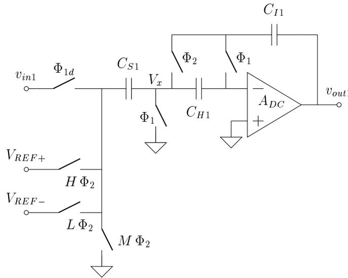
Figure 5.1: First integrator from the first stage of the MASH ADC
