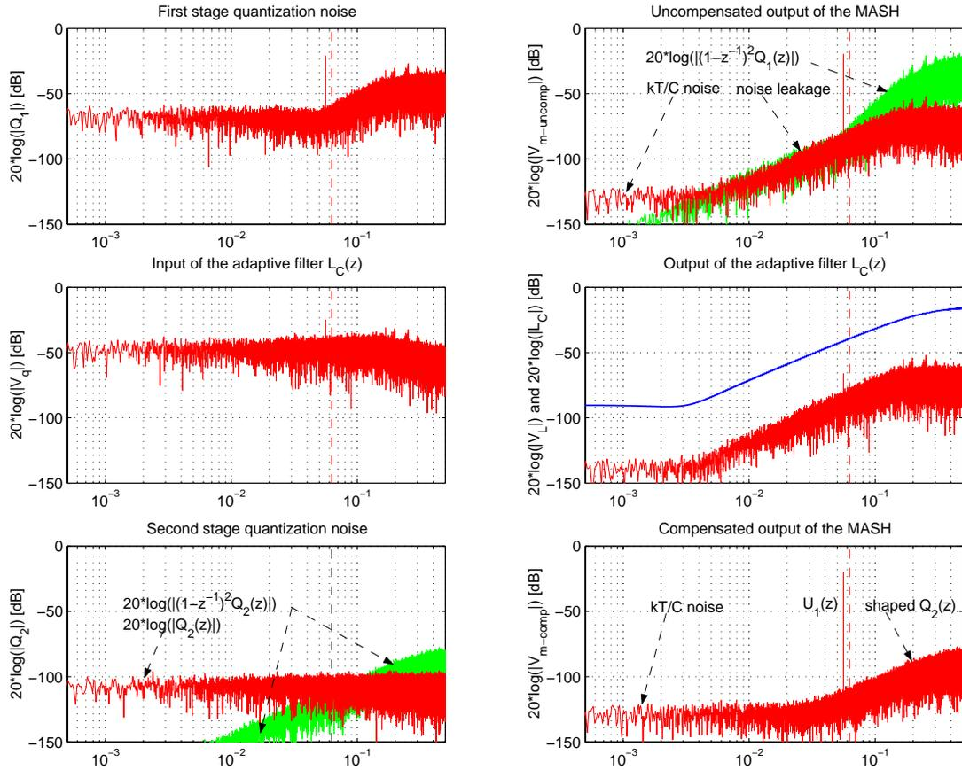
Figure 4.7: Spectral analysis of some internal / external signals of the MASH after a successful adaptive compensation process
