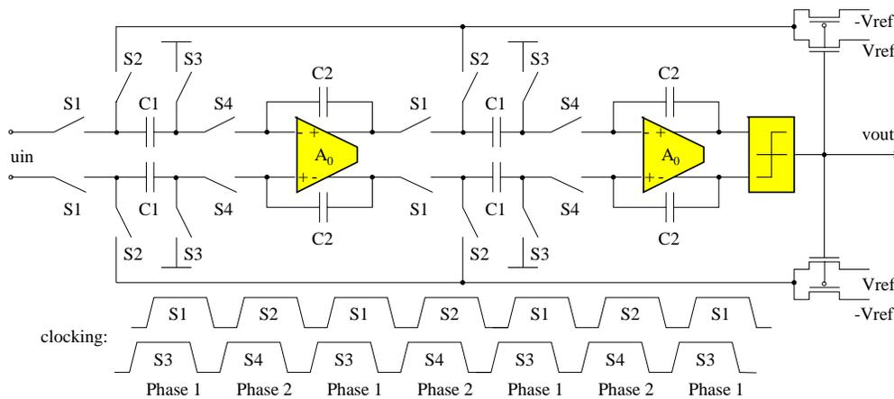
Figure 2.18: Switched-capacitor second-order delta-sigma ADC
