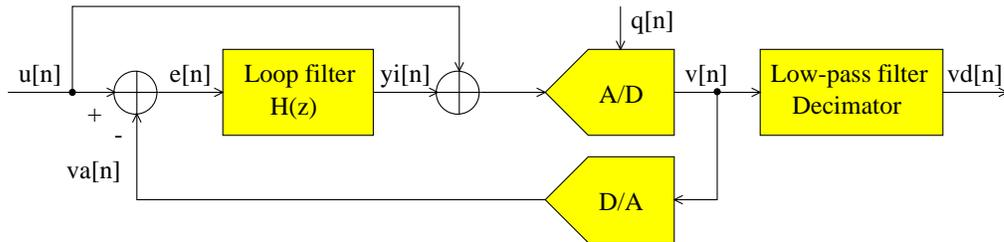
Figure 2.29: General delta-sigma modulator with a forward path
