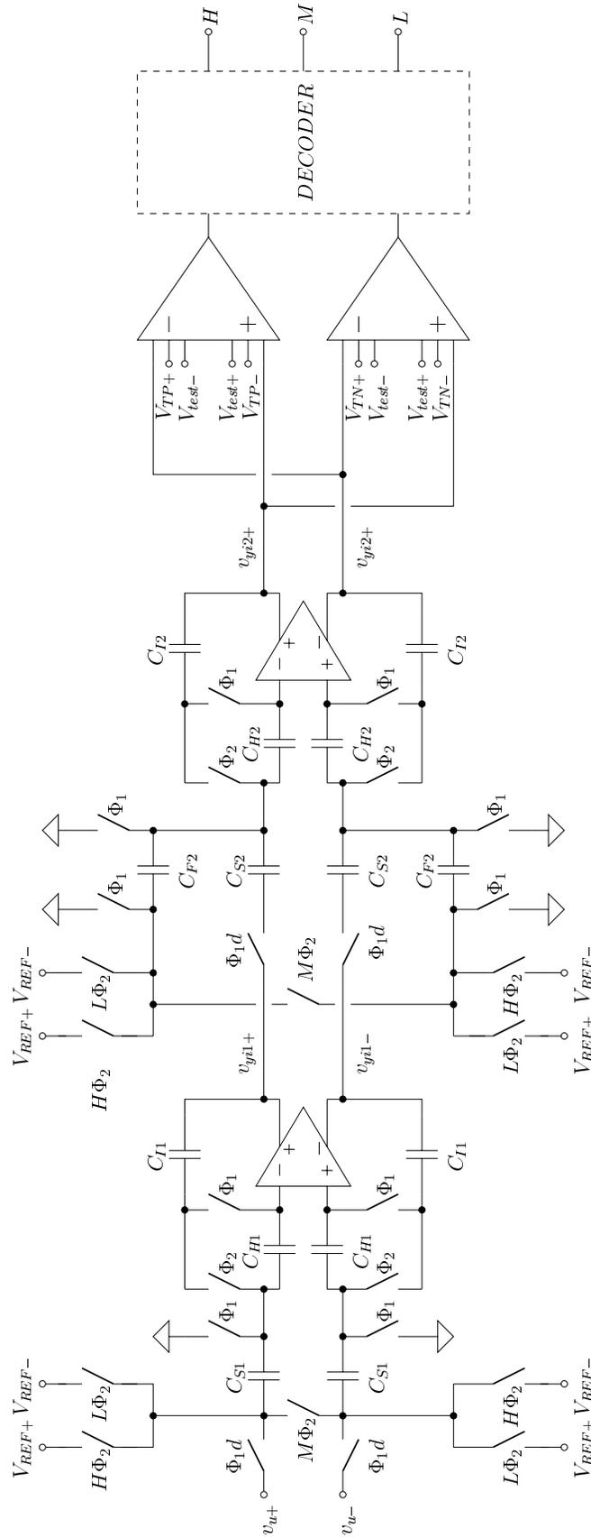
Figure 5.9: Detailed first stage (second-order 1.5-bit delta-sigma ADC) diagram
