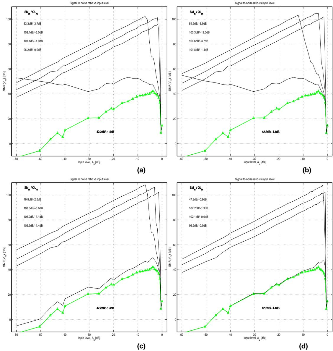
Figure 3.7: Comparative performance analysis between different ideal 2-0 MASH structures for  $OSR = 16$ ,  $N_1 = 1$  bit and  $N_2 = 12$  bits: (a) simplified structure,  $\beta = 1$ ,  $m_1 = 0$ ,  $m_2 = 2, 4, 8, 16$  (top to bottom); (b) improved standard structure,  $\beta = 0$ ,  $m_1 = 1$ ,  $m_2 = 1, 2, 4, 8$ ; (c) general structure,  $\beta = 2$ ,  $m_1 = -1$ ,  $m_2 = 1, 2, 4, 8$ ; (d) general structure,  $\beta = 4$ ,  $m_1 = -3$ ,  $m_2 = 2, 4, 8, 16$ .
