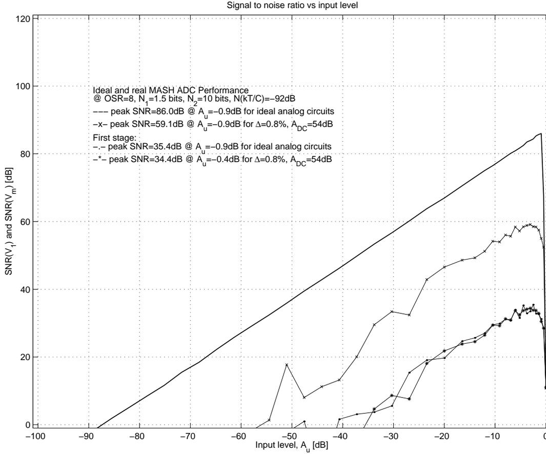
Figure 3.10: Ideal and real cascaded 2-0 delta-sigma ADC  $SNR$  performance ( $a_1 = \frac{1}{4}$ ,  $a_2 = \frac{1}{2}$ ,  $b_1 = 1$ ,  $b_2 = \frac{1}{2}$ ,  $k_1 = 8$ ,  $\beta = 2$ ,  $m_1 = -1$ ,  $m_0 = \frac{1}{2}$ ,  $m_2 = 2$ )
