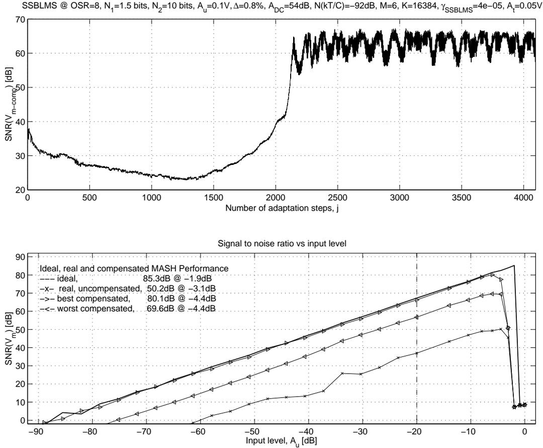
Figure 4.4: Adaptive compensation process and achieved  $SNR$  performance
