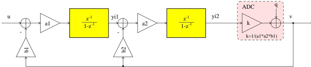
Figure 2.15: Linearized model of the second-order delta-sigma ADC
