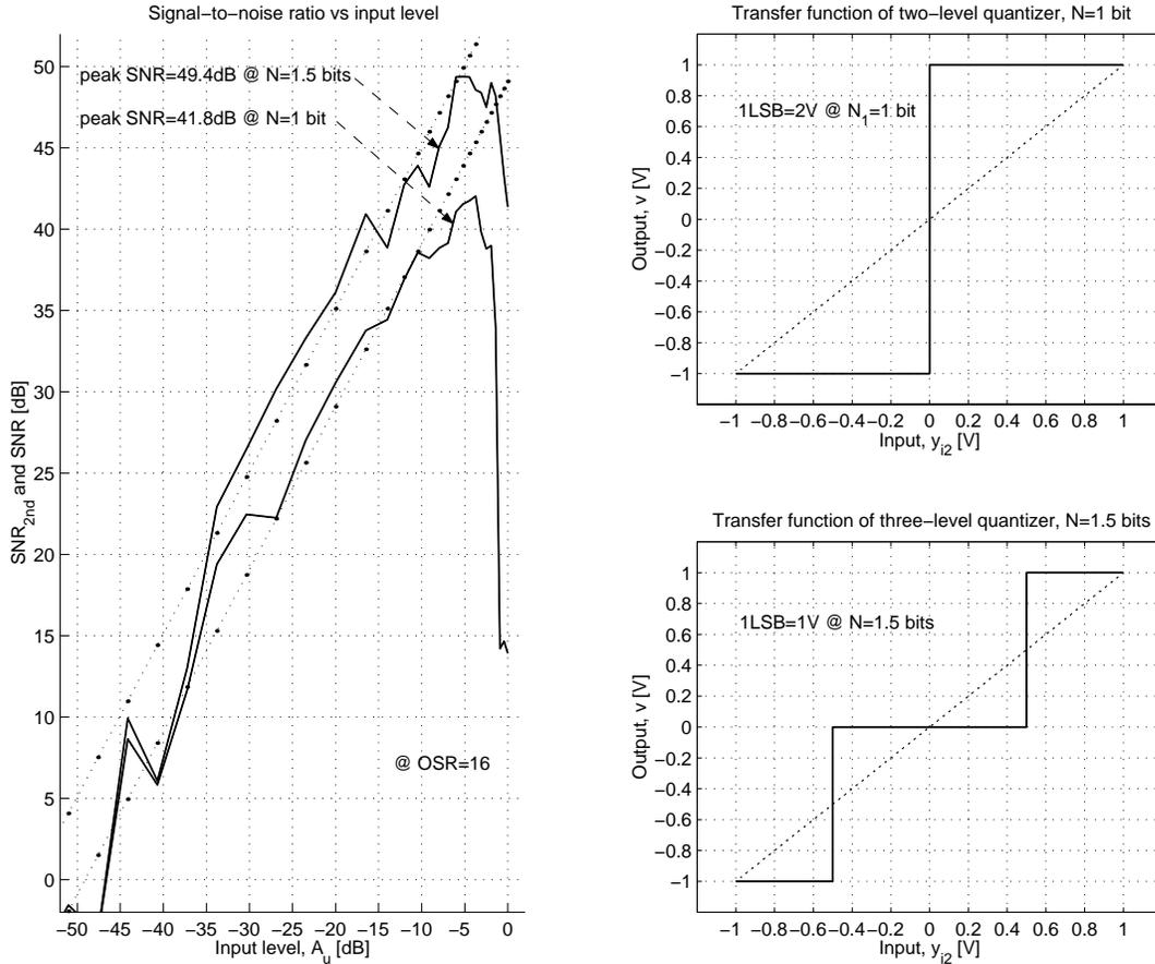
Figure 2.25: Comparative performance of bi- and tri-level modulators
