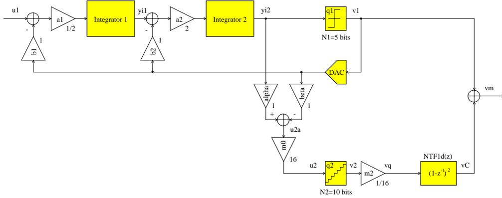
Figure 4.13: High-performance 2-0 MASH ADC
