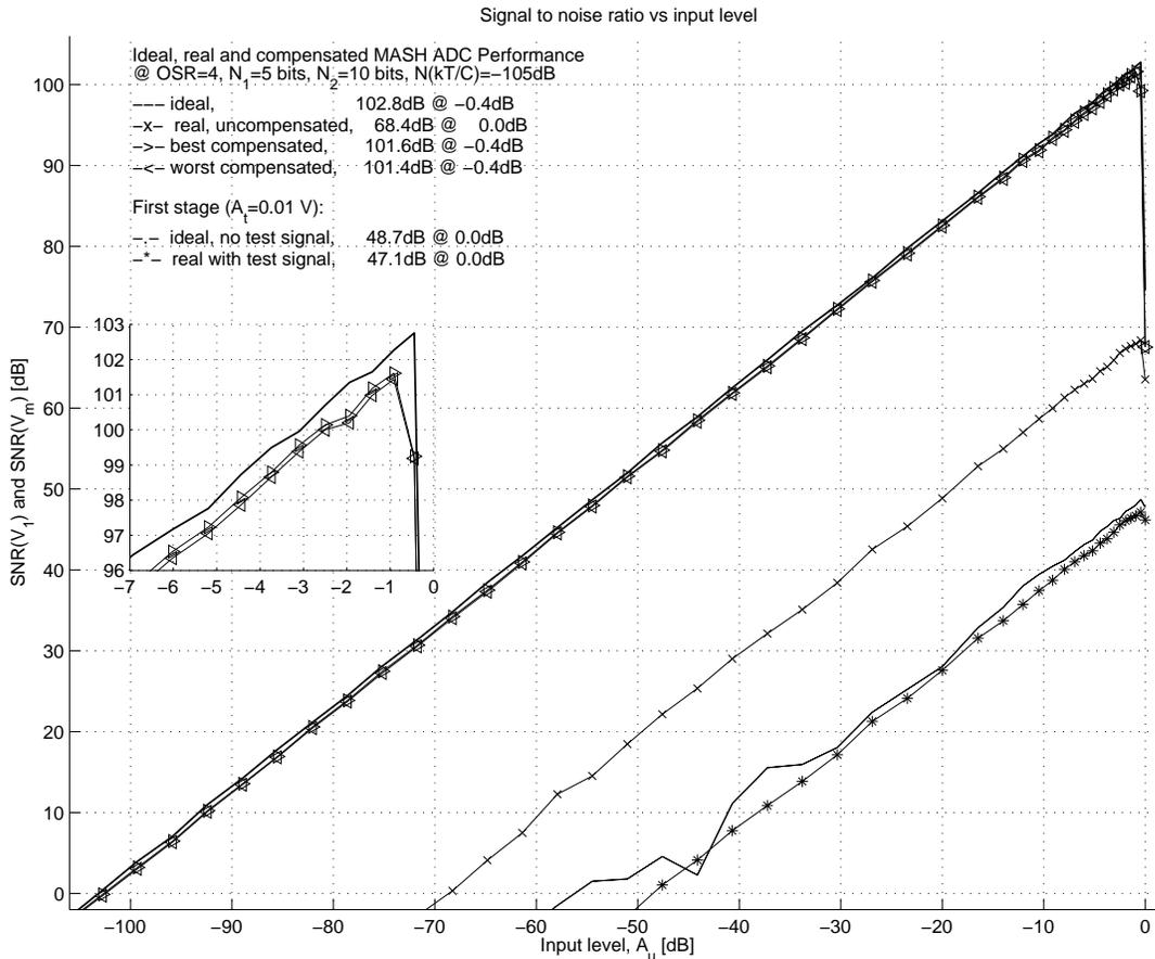
Figure 4.14: Simulated  $SNR$  performance of the high-performance 2-0 MASH ADC ( $f_S = 100$  MHz,  $OSR = 4$ ,  $N_1 = 5$  bit,  $N_2 = 10$  bit,  $A_{DC} = 54$  dB, and  $\Delta_C = 0.4\%$ )
