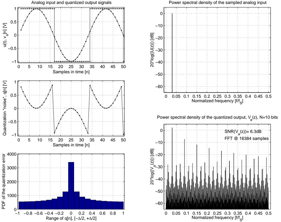
Figure 2.9: The spectrum of a quantized sinewave for  $N=1$  bit
