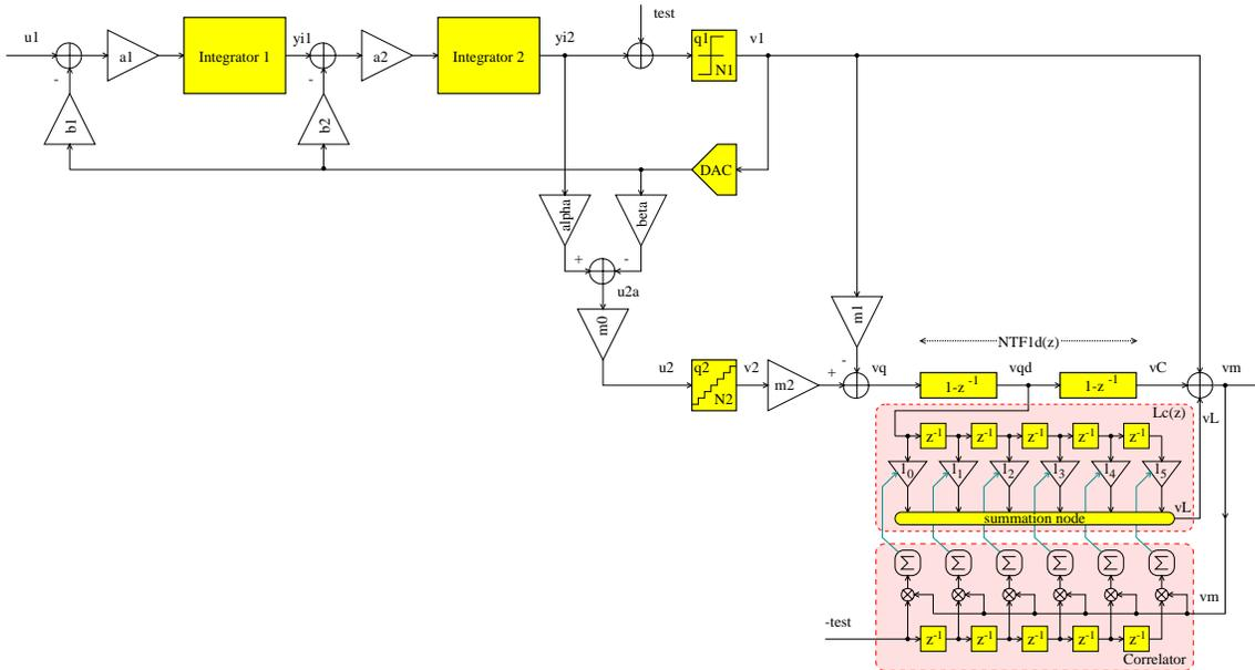
Figure 4.8: Improved adaptive digital noise-leakage compensation scheme using a test signal  $test[n]$  for the general cascaded 2-0 delta-sigma ADC
