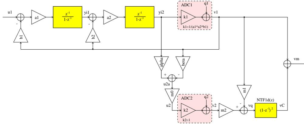
Figure 3.6: Linearized model of the general cascaded 2-0 delta-sigma ADC
