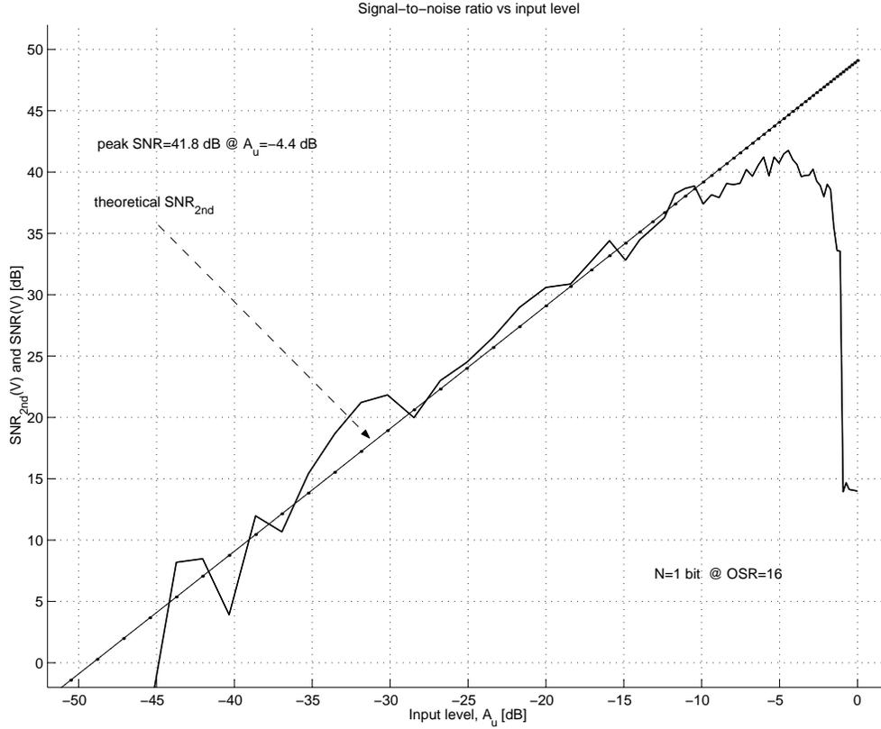
Figure 2.21: Performance of the second-order single-bit delta-sigma ADC
