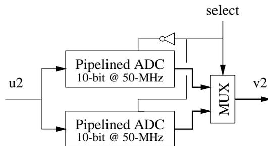
Figure 5.11: Time-interleaved 2 pipelined ADC implementing the second-stage quantizer
