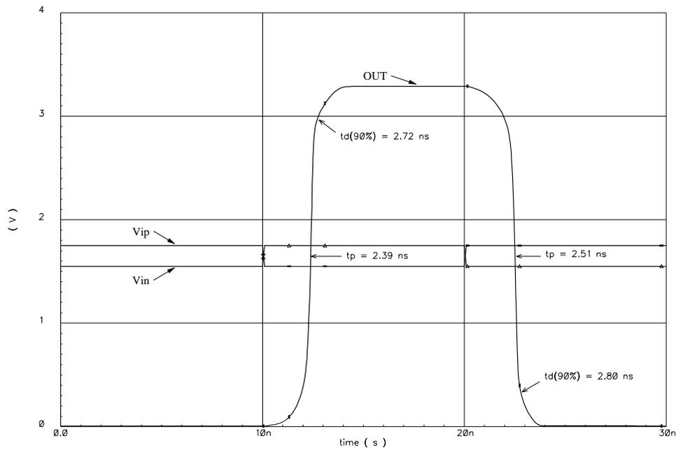
Figure 5.16: Response of the comparator to a step
