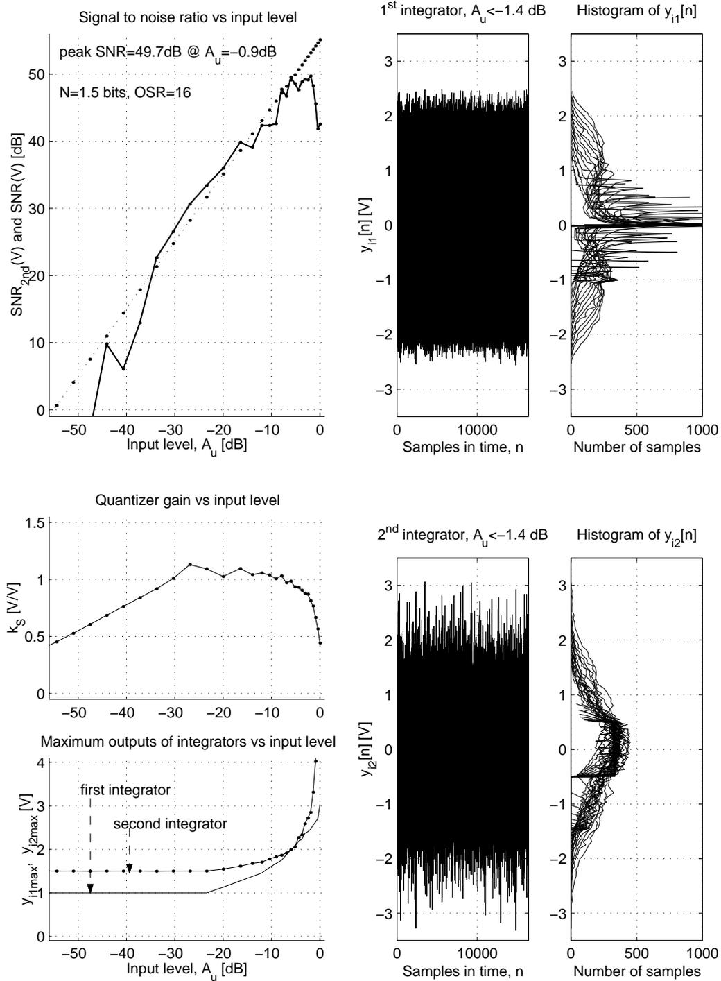
Figure 2.27: Internal voltage swings for  $a_1 = 1, a_2 = 1, b_1 = 1, b_2 = 2, k = 1$
