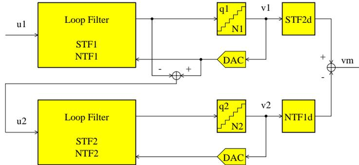
Figure 3.1: General structure of a cascaded delta-sigma modulator
