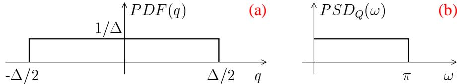
Figure 2.4: Statistical properties of the quantization error as input-independent additive white noise: (a) probability density function  $PDF(q)$  and (b) power spectral density  $PSD_Q(\omega)$
