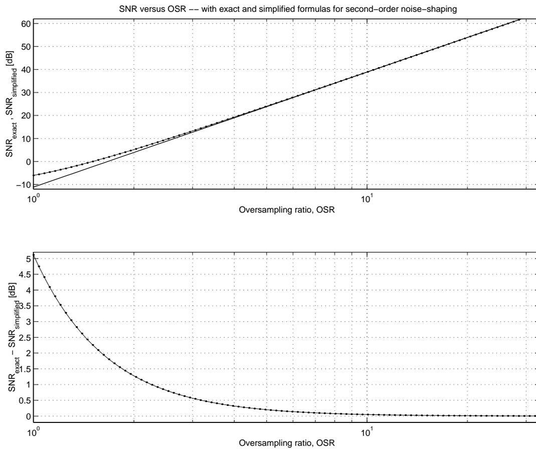
Figure 2.17: Signal-to-noise ratio  $SNR$  versus oversampling ratio  $OSR$
