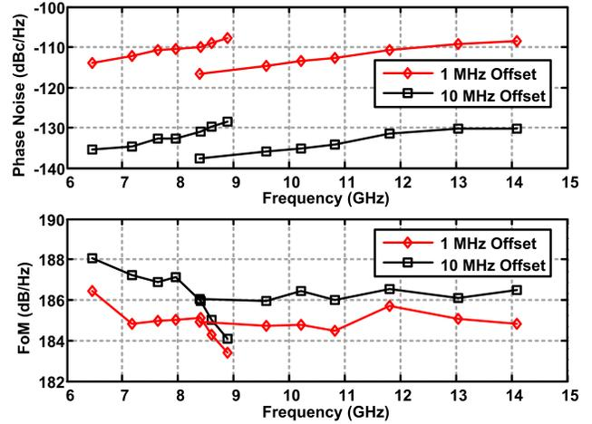
Fig. 10. Measured dual-mode VCO phase noise and FoM.
