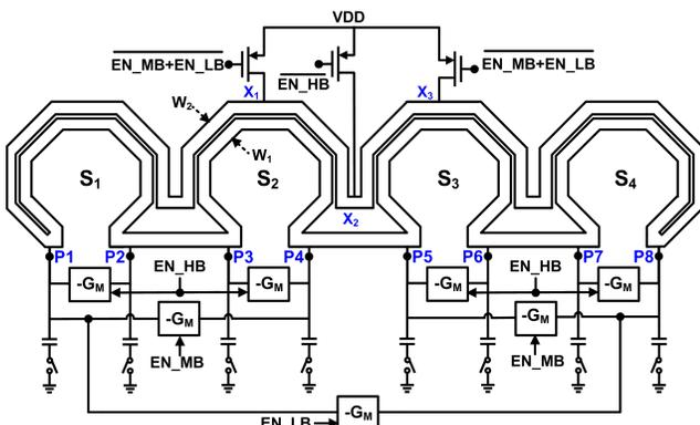
Fig. 5. Schematic of a 2.2GHz-8.7GHz VCO that extends the proposed series resonant mode-switching approach to 3 modes.
