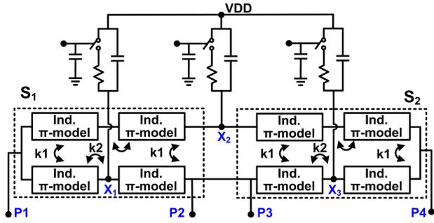
Fig. 4. Broadband inductor model to evaluate impact of supply-switch parasitics on VCO.
