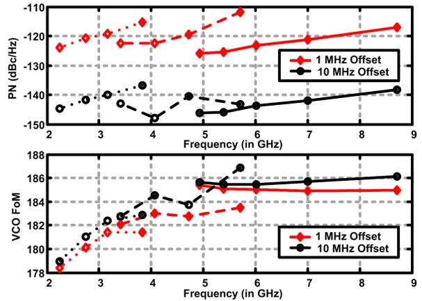
Fig. 7. Measured triple-mode VCO phase noise and FoM.
