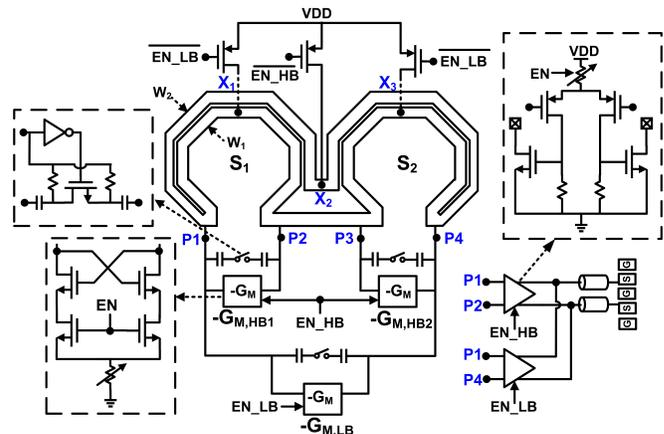
Fig. 1. Schematic of proposed series resonator mode-switching CMOS VCO with octave tuning range (6.39GHz to 14GHz).
