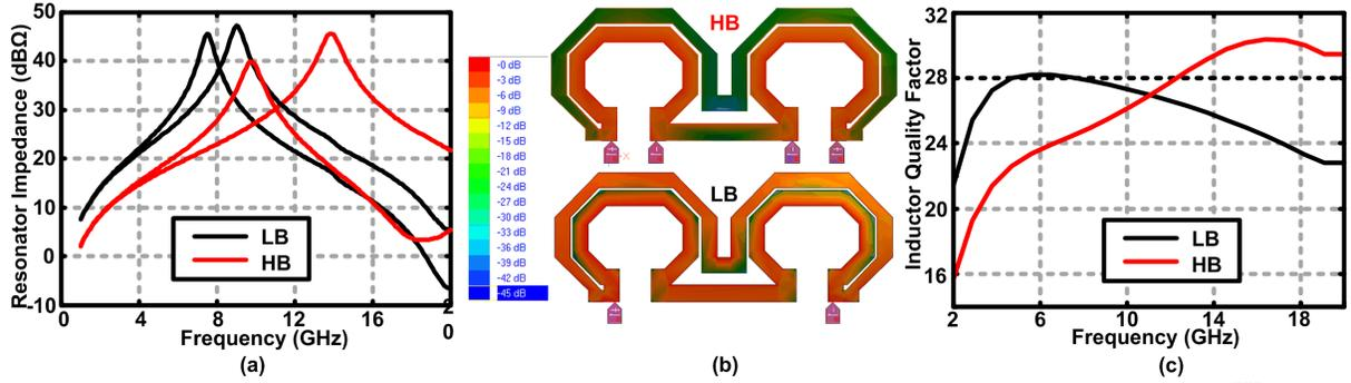
Fig. 2. (a) Simulated resonator impedance in HB and LB modes, (b) Current distribution in inductor structure -  $W_2$  carries less current than  $W_1$  in HB Mode, while the effective width is  $W_1 + W_2$  in LB mode [6], (c) Simulated inductor  $Q$  in LB and HB modes.
