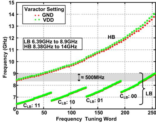
Fig. 8. Measured dual-mode VCO FTR (500MHz band overlap).
