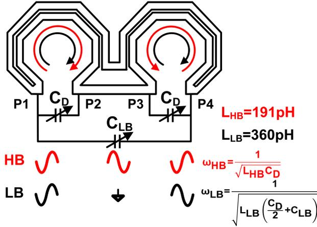
Fig. 3. Resonator properties in HB and LB modes for series resonator mode-switching.
