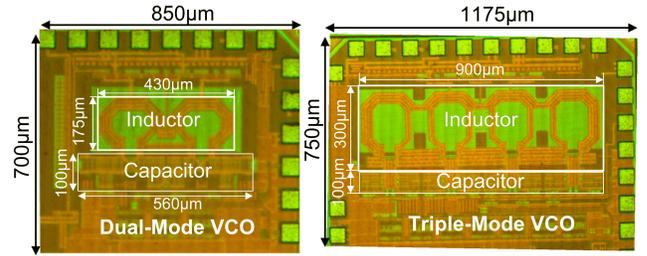
Fig. 6. Die photo of dual-mode (6.4GHz-14GHz) and triple-mode (2.2GHz-8.7GHz) VCO.
