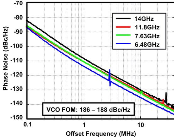
Fig. 9. Measured VCO phase noise across offset frequency.
