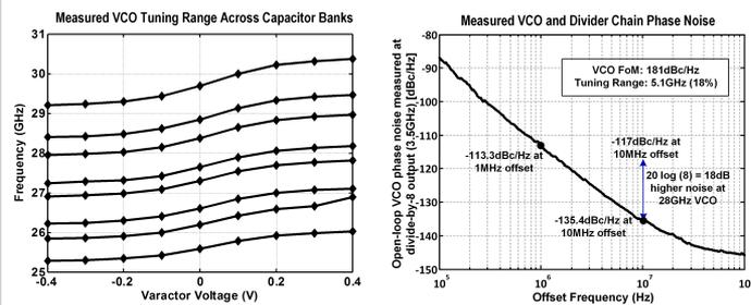
Figure 2.2.4: Measured 28GHz-VCO tuning range across switched capacitor banks and measured open-loop VCO phase noise.
