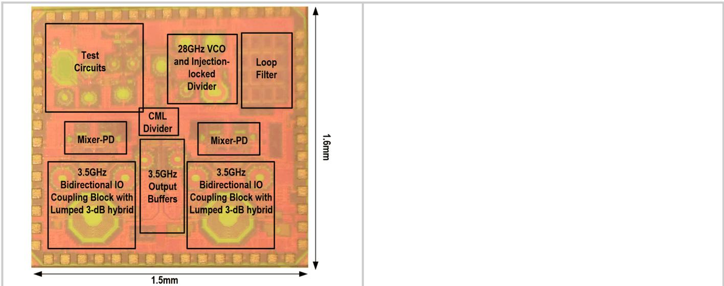
Figure 2.2.7: Die micrograph of the single-wire scalable 28GHz coupled PLL.
